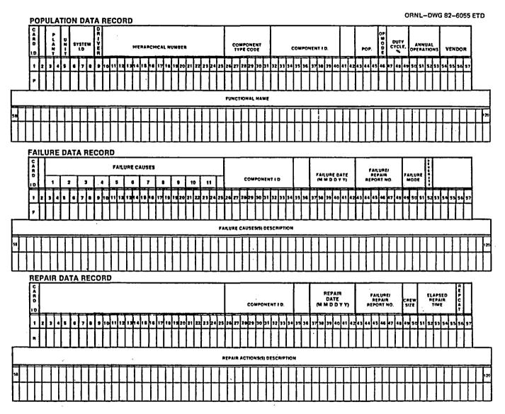
Fig. 2.1. IPRD population, failure, and repair data record forms for pumps.
