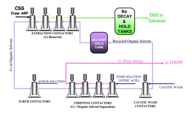
Figure 2.7: Modular CSSX Unit Process
