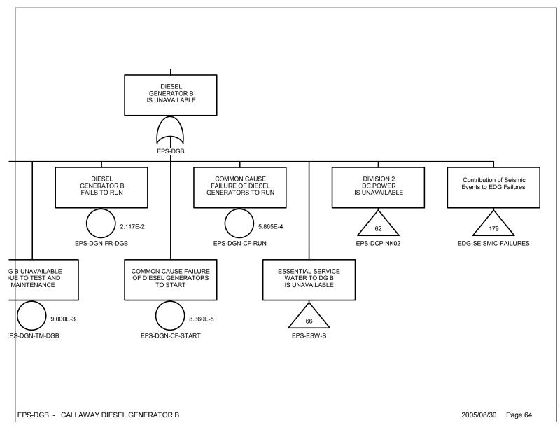
Figure 4-7 Adding Seismic Failures to a Support System - Figure 2 of 3
