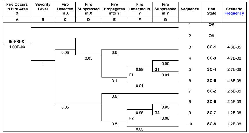
Figure 2A-2-1 An Example Event Tree Model with Possible Propagation
