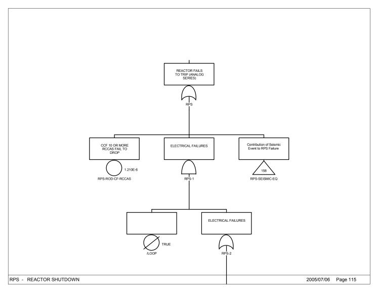
Figure 4-4 RPS Fault Tree (partial top showing introduction of seismic faults)
