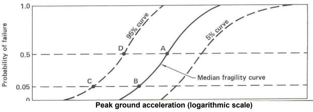
Figure 4C-1 Fragility Curves. Peak ground acceleration corresponding to Point A represents the median capacity. Peak ground acceleration corresponding to Point C represents the HCLPF capacity.
