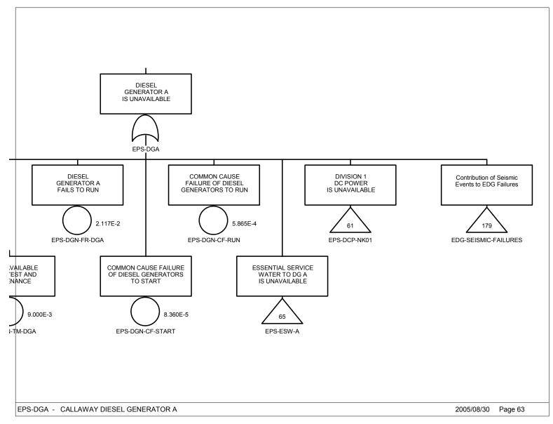
Figure 4-6 Adding Seismic Failures to a Support System - Figure 1 of 3
