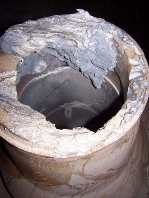
Surge nozzle after initial prep work (note ID damage caused by flame cutting)
