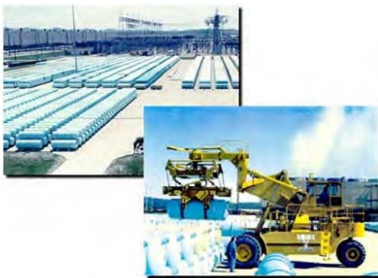
Figure 1- 3 UF_6 Cylinders Stored at the Paducah Gaseous Diffusion Plant
