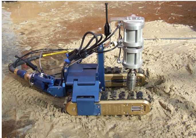
Figure 5.2-7: Robotic Sampler at Test Facility
