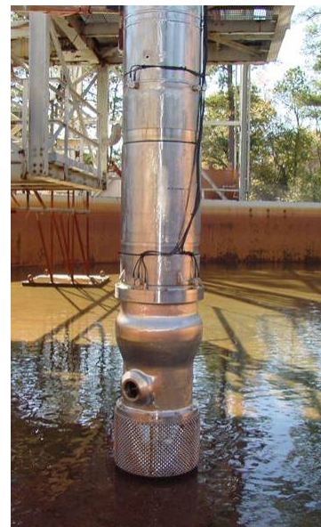
Figure 2.3-4: Submersible Mixing Pump in a Test Tank
