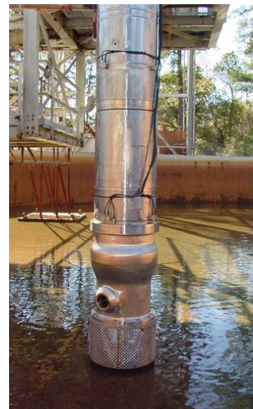
Figure 5.2-4: Submersible Mixing Pump in a Test Tank
