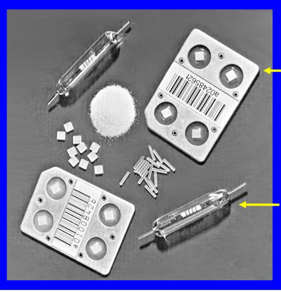
Four LiF chips sandwiched between two sheets of Teflon and mounted on an aluminum card/holder with barcode.
