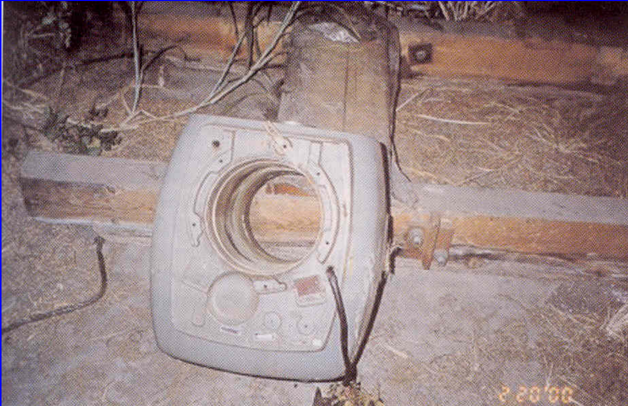
Teletherapy Head with Source Drawer Missing
