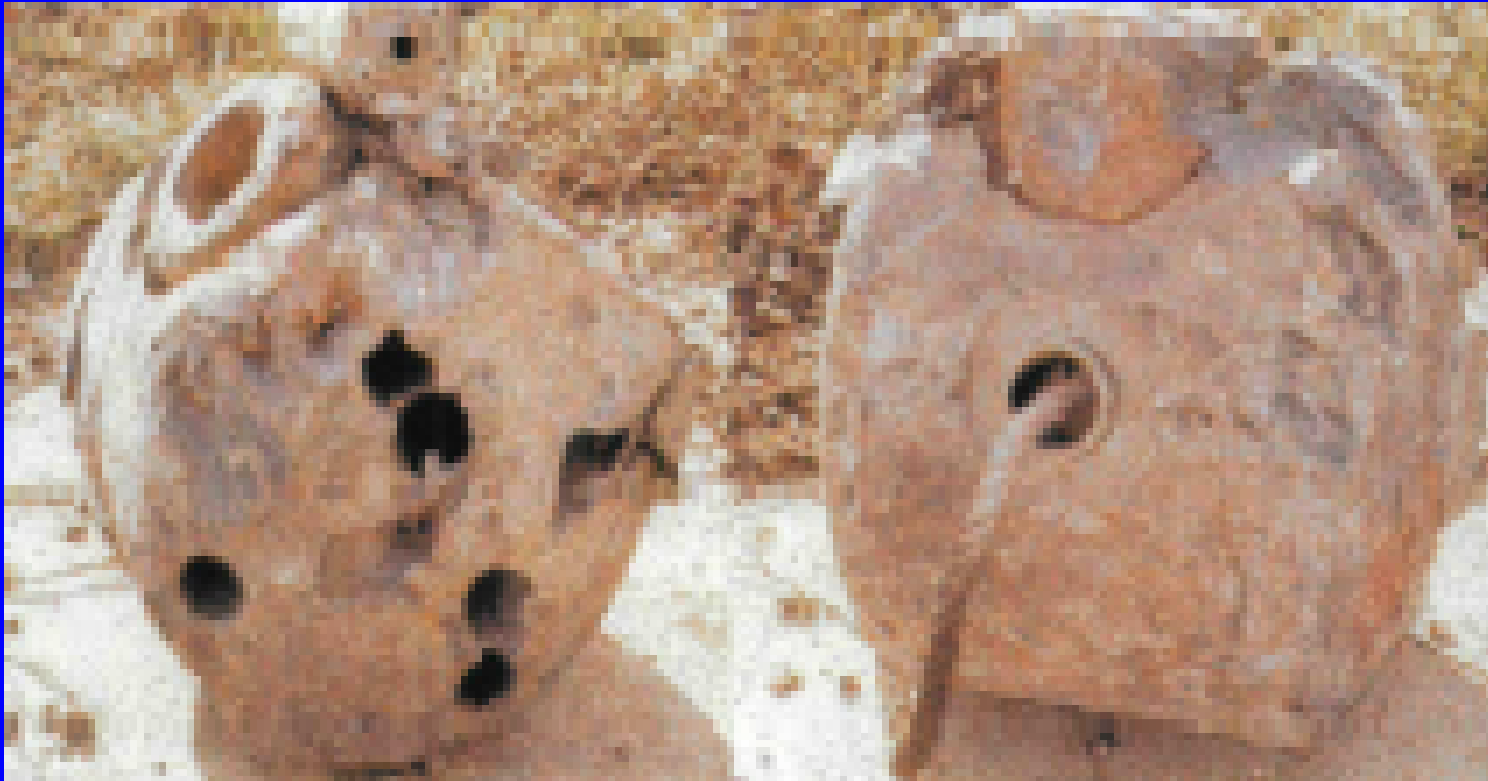
Damaged source exchange containers
