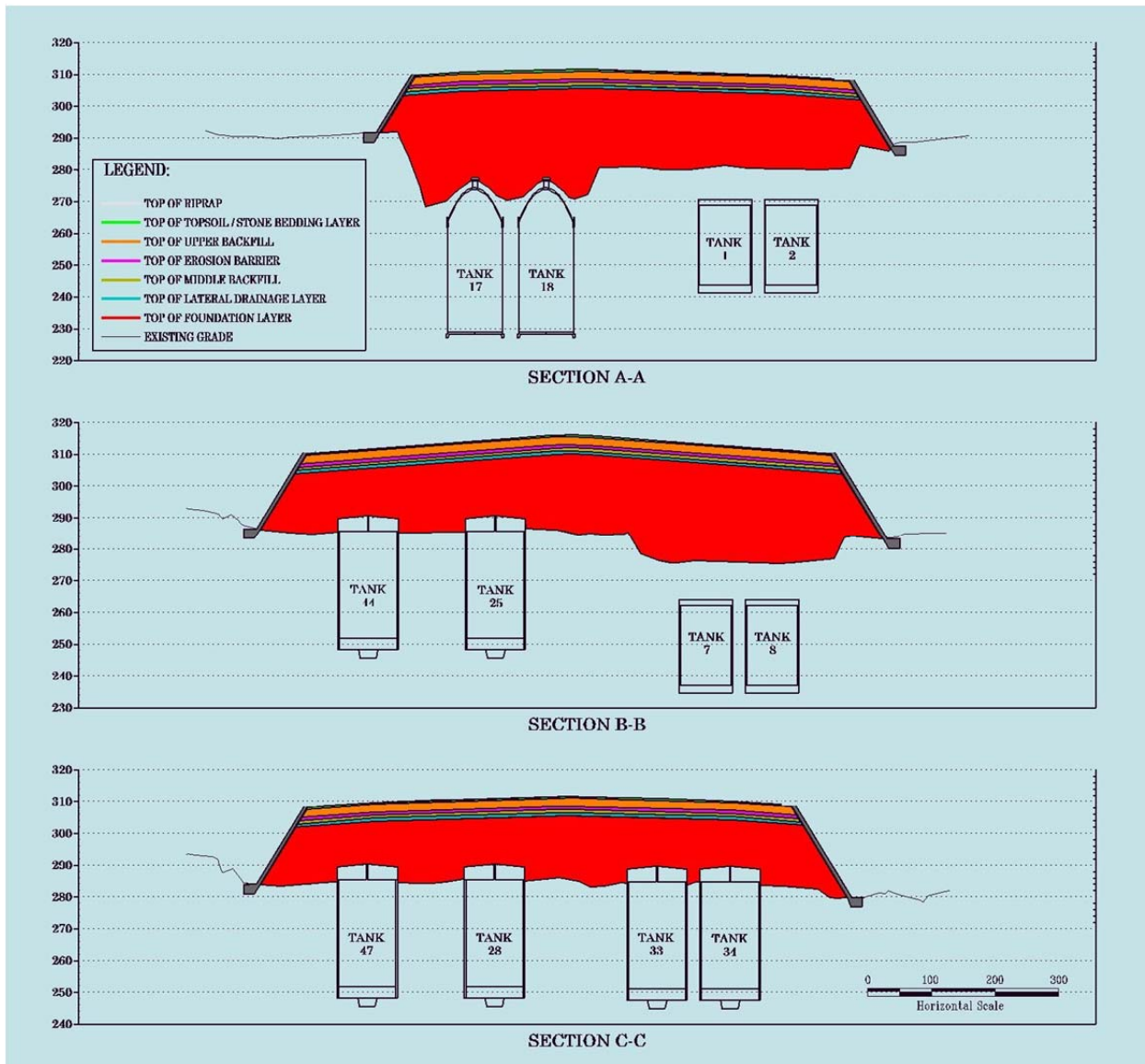
Figure 2.6-3: FTF Closure Cap Conceptual Design, Sections A-A, B-B and C-C
