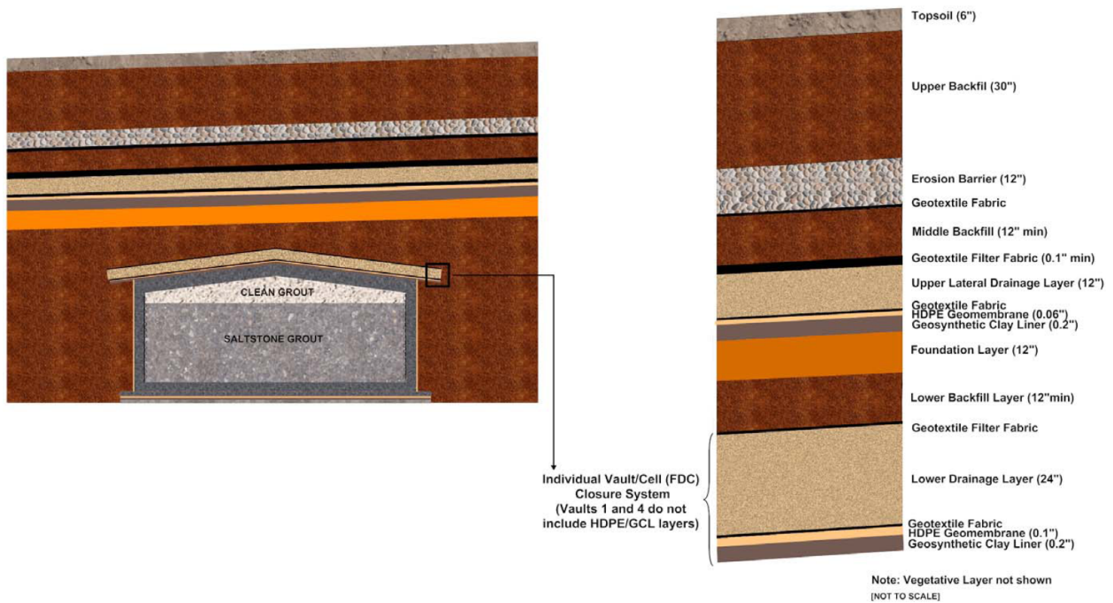
Figure 2.4-2: Conceptual illustrations of the components of the SDF closure caps and additional engineered layers above the disposal units (2009 PA; Figure 3.2-20)
