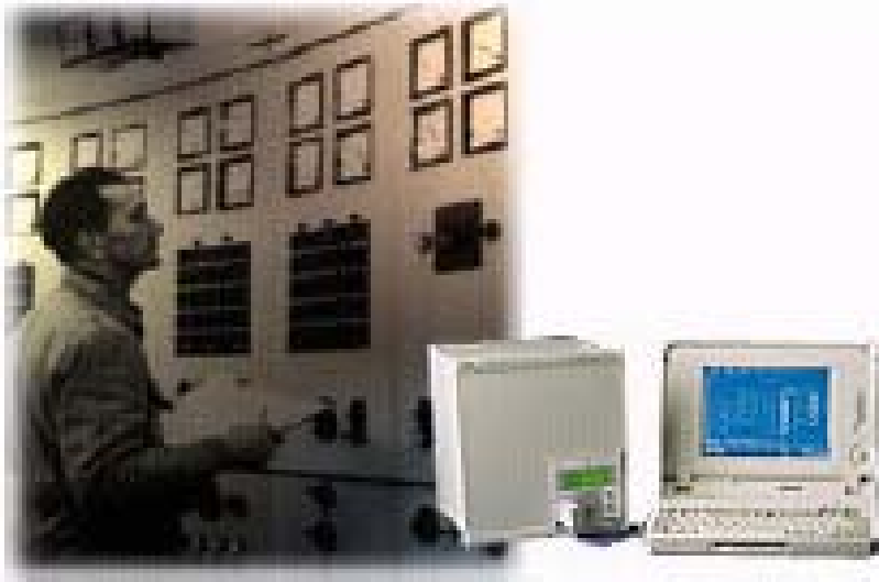
Figure 1-61 Comparison of Protective Relaying Equipment from 1925 and 1994
