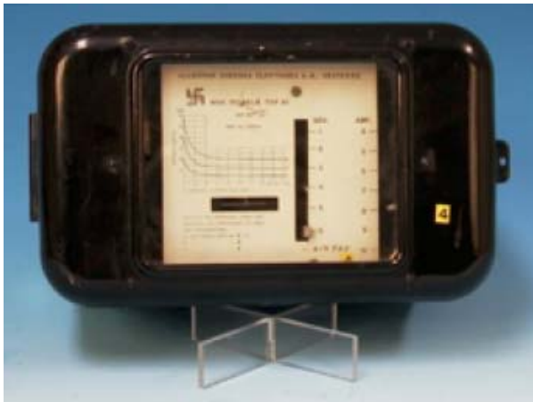
ABB Induction Type Time Overcurrent Relay 1920 – 1985
