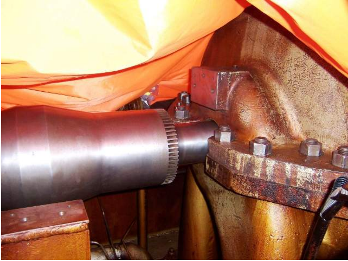
Figure 1-48 New Speed Pickup Gear
