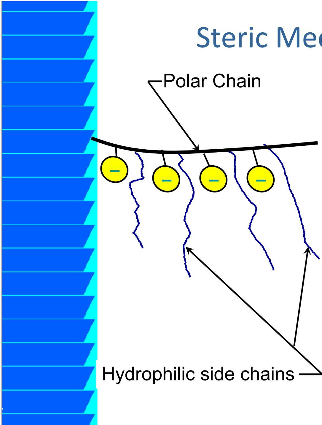
Unlike traditional superplasticizers, molecules of polycarboxylate consist of ether with a very flexible polar chain carrying negative functional groups and long hydrophilic side chains
