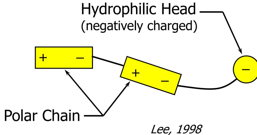
Water Reducers are typically hydrophilic surfactants which consist of a polar chain and a negatively charged head.
