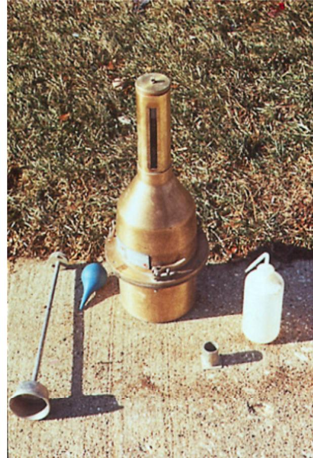
Volumetric Method – ASTM C173
