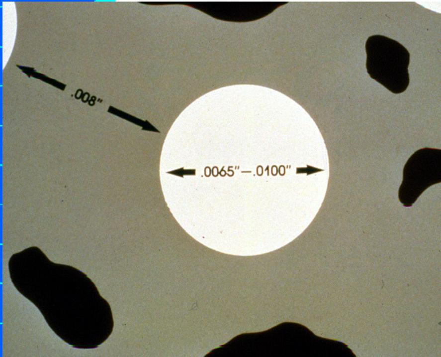
Spacing Factor and Specific Surface are More Important than Total Volume (%) of Air
