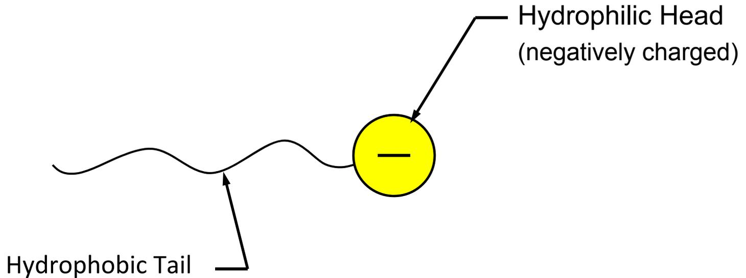
Air-Entraining Admixtures are typically surfactants that have a negatively charged head which is hydrophilic, and a hydrophobic tail.
