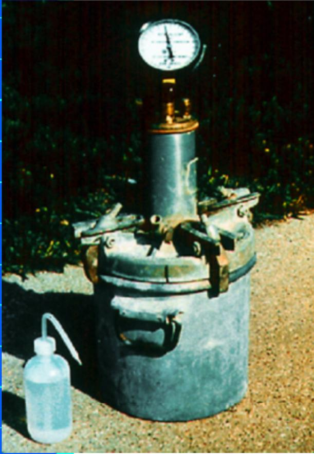
Pressure Method – ASTM C231
