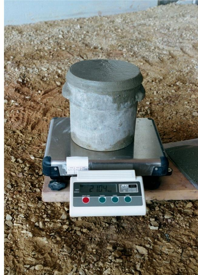
Gravimetric Method – ASTM C138
