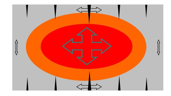
Crack width is a function of the temperature difference
