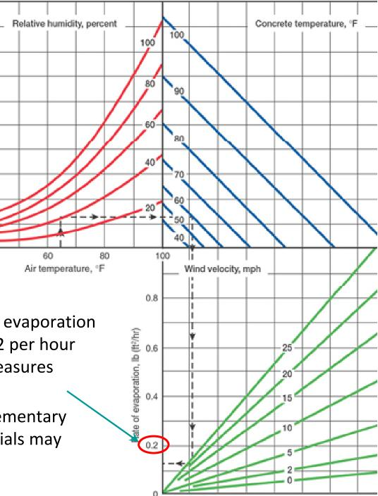
When the rate of evaporation exceeds 0.2 lb/ft2 per hour precautionary measures should be taken.
