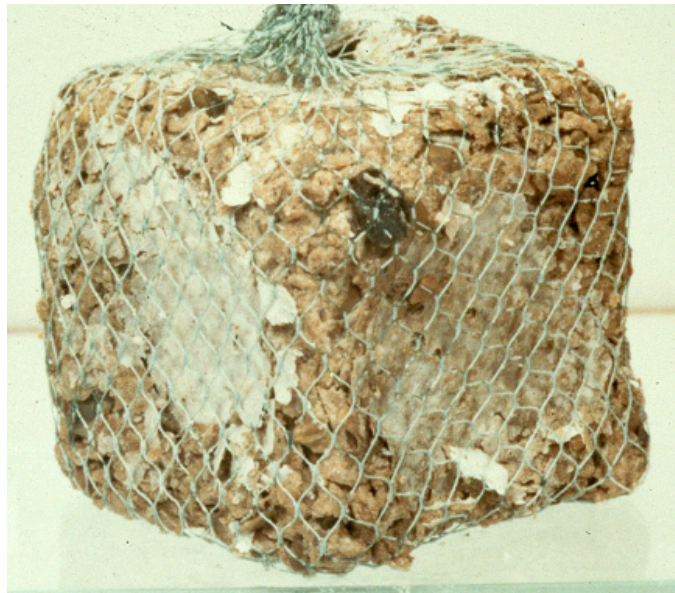
After immersion in sulfate solution for 5 years
