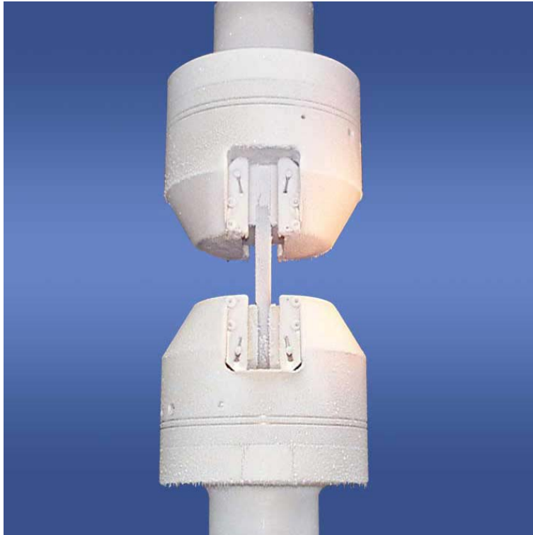
Test coupon in the loading grips
