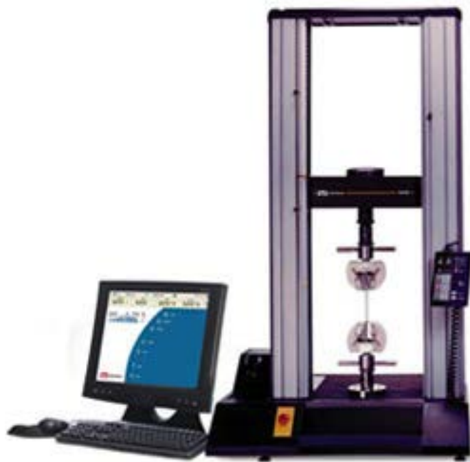
Modern Loading System - Computer Controlled
