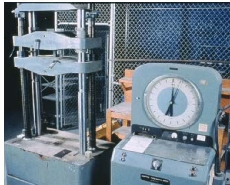
Conventional Loading System – for Tensile Strength Only
