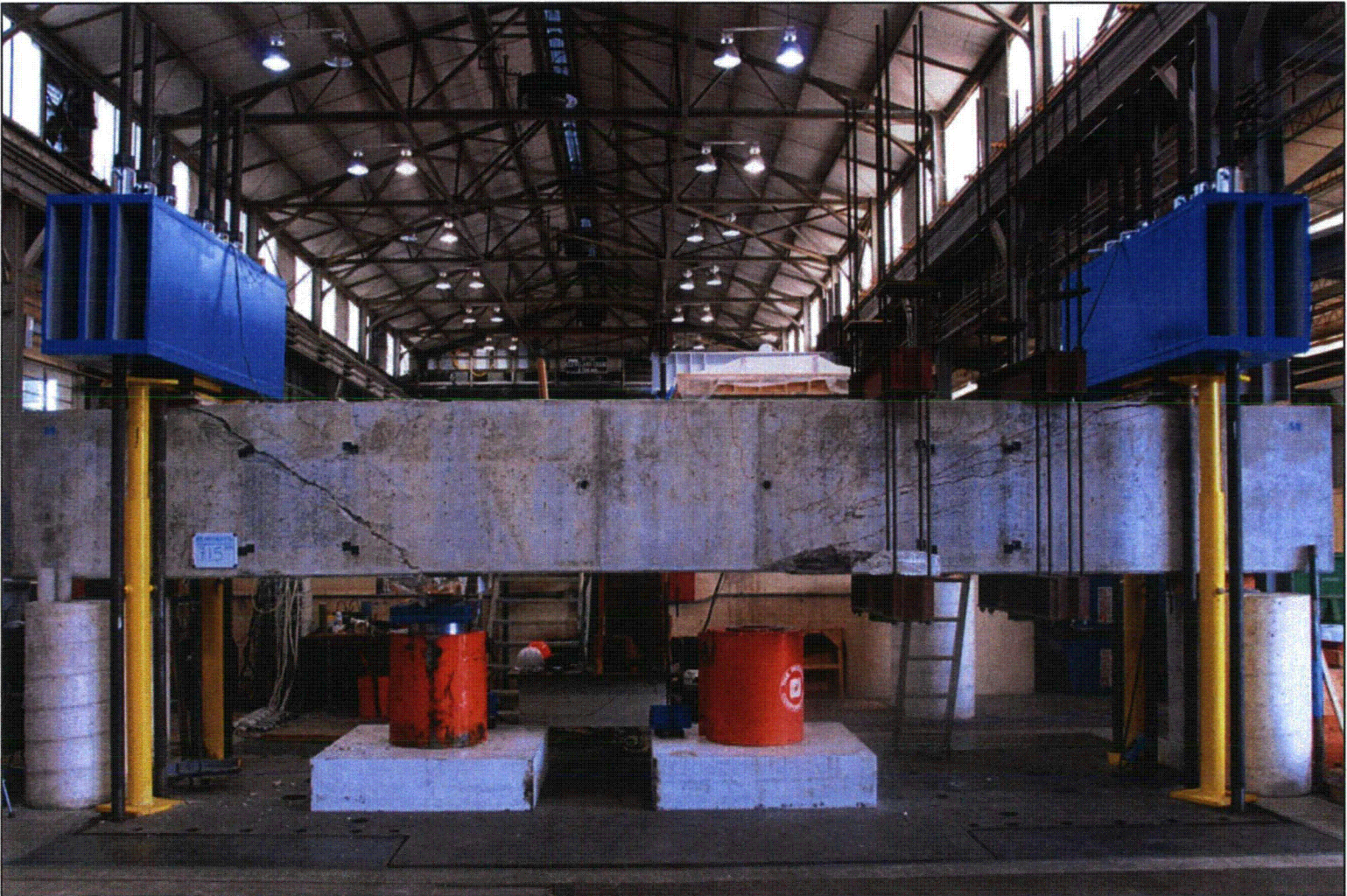
Figure 6: Large-Scale Beam Test Facility Configured for Shear-Dominated Testing
