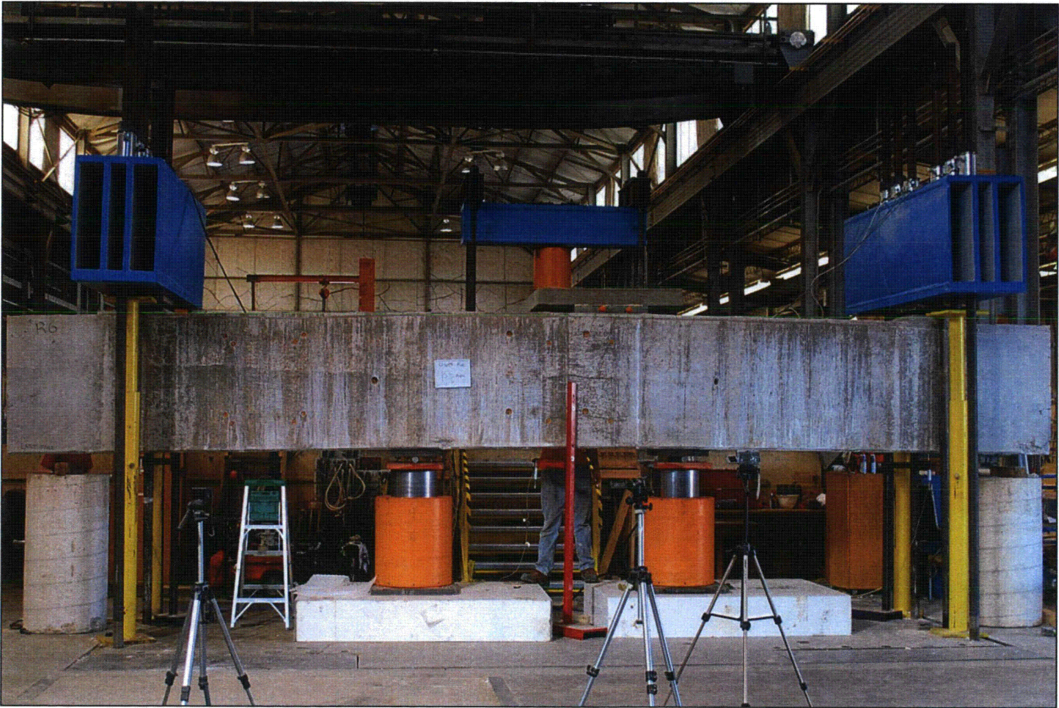
Figure 7: Large-Scale Beam Test Facility Configured for Flexure-Dominated Testing
