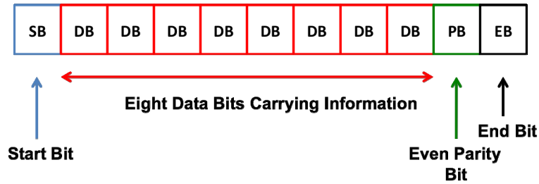
Figure 4-6 X-bus transmission packet (PTP)
