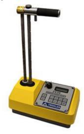
A typical moisture-density gauge is shown above.
