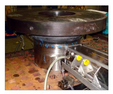
Figure 9.12 Pressurizer surge nozzle DM weld mockup being measured for WRSs
