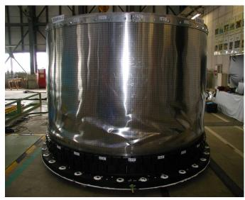
Figure 12.16 JNES Ultimate Strength Test of Cylindrical Liquid Storage Tanks Subjected to an Earthquake
