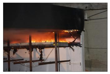
Figure 7.8 Burning cables in hallway enclosure (end view of burning cables in two horizontal trays in hallway enclosure)
