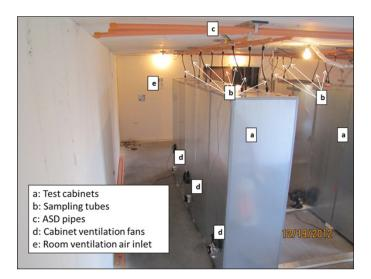
Figure 7.19 Fire test room configuration
