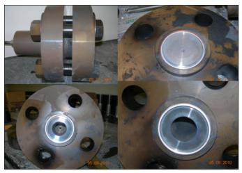
Figure 7.15 Pictures of the small-scale test vessel after 800 degrees C exposure for 9 hours (small-scale test vessel [top left], vessel head after disassembly [top right], and vessel body and metallic seal after disassembly (bottom left and bottom right])
