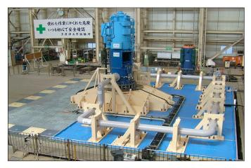
Figure 12.15 JNES seismic fragility test of large vertical shaft pump
