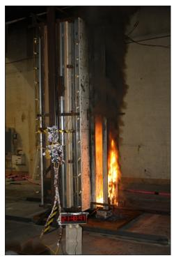
Figure 7.7 Burning cables in vertical trays (side view of burning cables in two vertical trays after ignition using a small gas burner)
