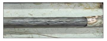
Figure 7.13 Photo of Kerite-FR cable after testing, showing the cracking of insulation material
