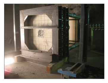
Figure 12.11 Impact of hard missile on prestressed concrete wall
