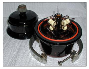
Figure 3.3 BIP irradiation vessel with sample coupons
