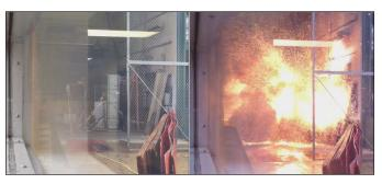
Figure 7.22 480 V load center undergoing HEAF testing: before arcing (left); after arcing (right)
