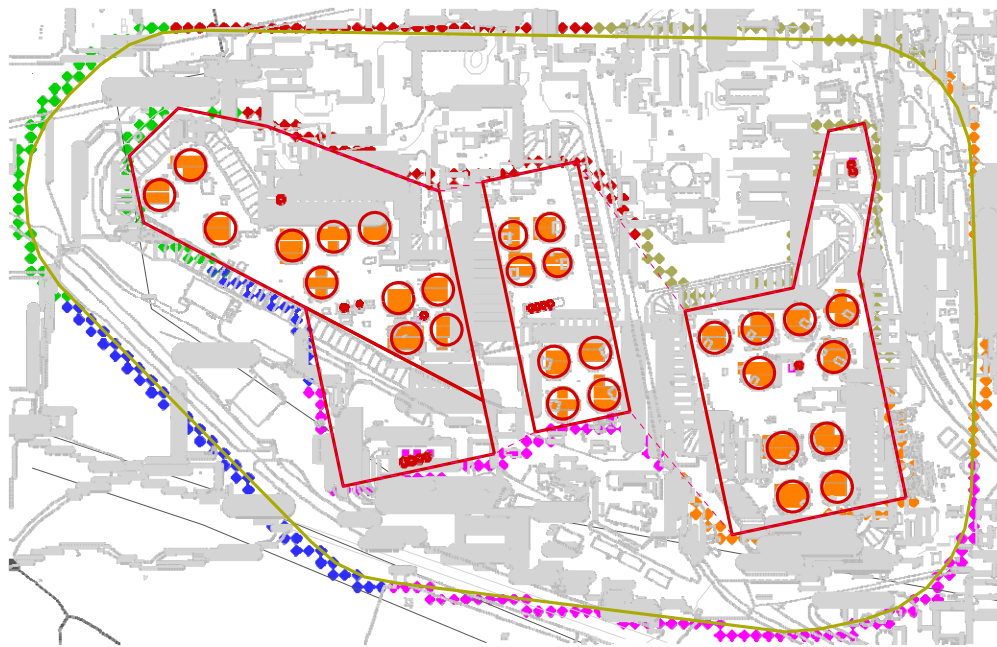
Figure 4-3 HTF/PORFLOW™ Saturated Zone Model Domain Showing Both Discrete and Distributed Sources, Stream Traces from Waste Tank Sources, and 1-m (3-ft) and 100-m (330-ft) Compliance Evaluation Sectors (A–F)
