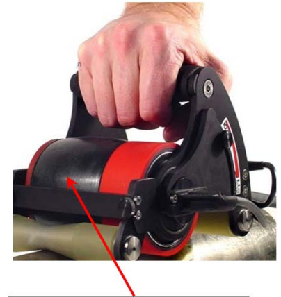
2-in wide array of 64 ultrasonic elements
