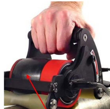
2-in wide array of 64 ultrasonic elements
