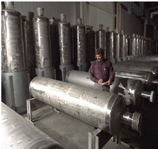
Figure A.3-1: Vitrification Canister Prior to Use
