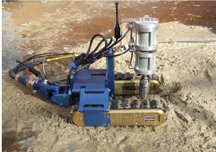
Figure 5.2-7: Robotic Sampler at Test Facility
