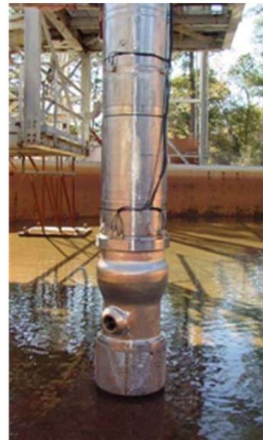
Figure 5.2-5: Submersible Mixing Pump in a Test Tank
