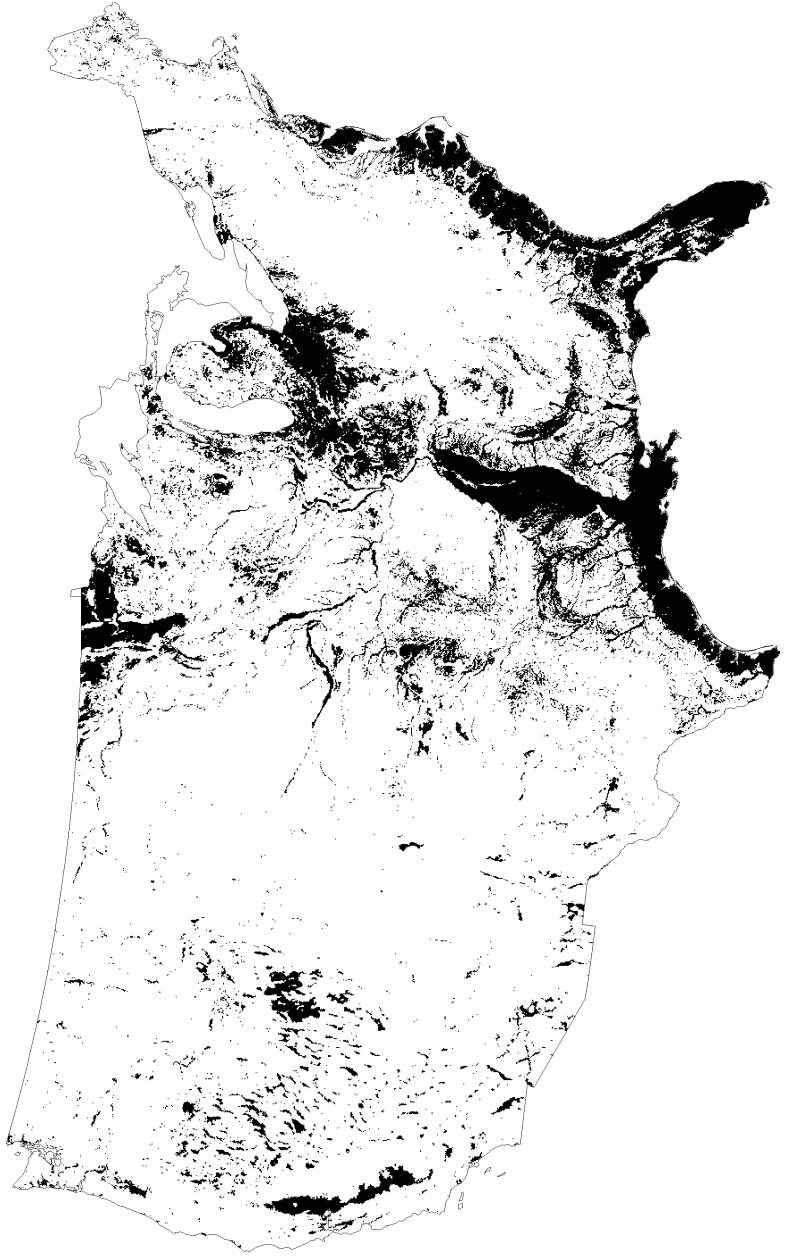
Figure B-4: Approximate area of simulated current water tables shallower than 30 m. Proposed sites located in these areas may require additional site characterization and analysis. Future near-surface groundwater areas may change (Kreakie et al, 2012)
