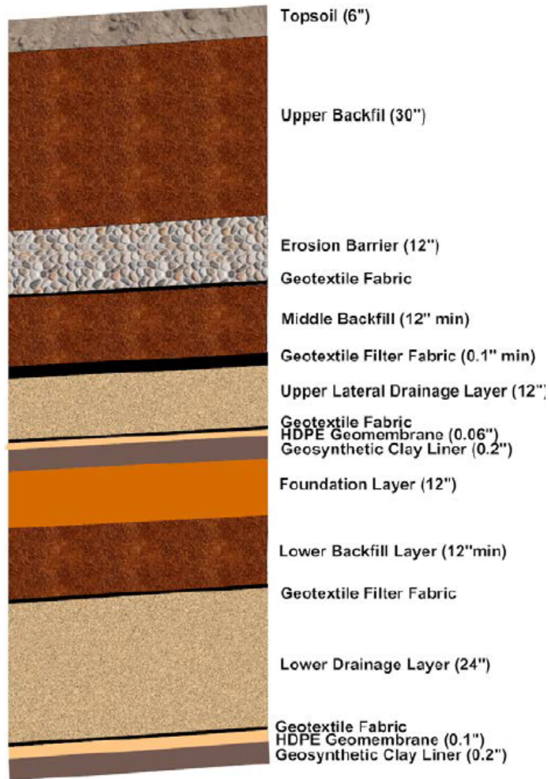
Figure 1: Layers of the SDF Conceptual Cover (Right-Side of Figure 3.2-20 in SRR-CWDA-2009-00017, Rev. 0)
