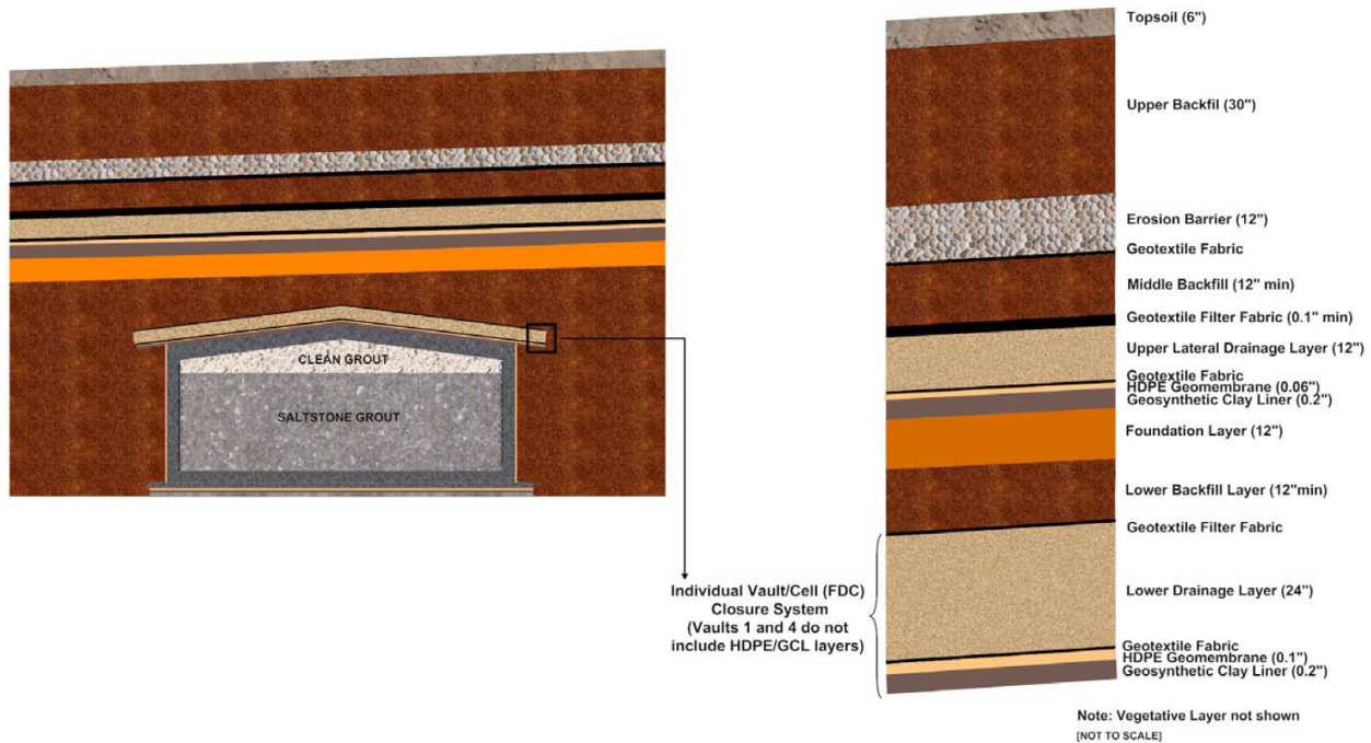
Figure 1: Conceptual illustrations of the components of SDF engineered cover (Figure 3.2-20 in SRR-CWDA-2009-00017, Rev. 0)
