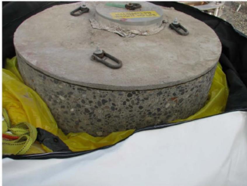
Figure 6-14. Evaluation of 55-inch Diameter Reinforced Concrete Dome Plug from Tank 214-C-107.
