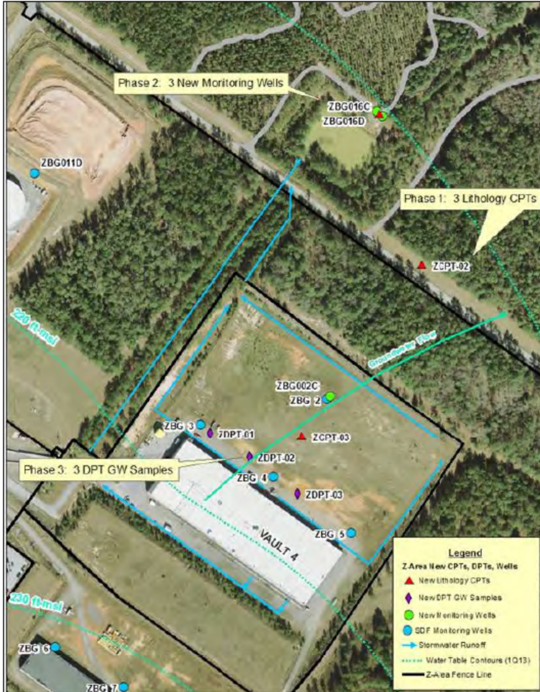
Figure 4: SDS 4 and Drainage Path to Sedimentation Basin 4 near Well ZBG 16C and Well ZBG 16D (from SRR-CWDA-2014-00054)
