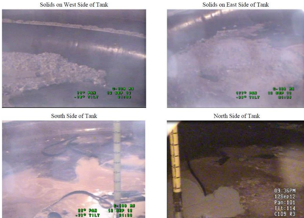
13 Figure 4-20. Photographs of Tank C-109 at Completion of Caustic Cleaning.
