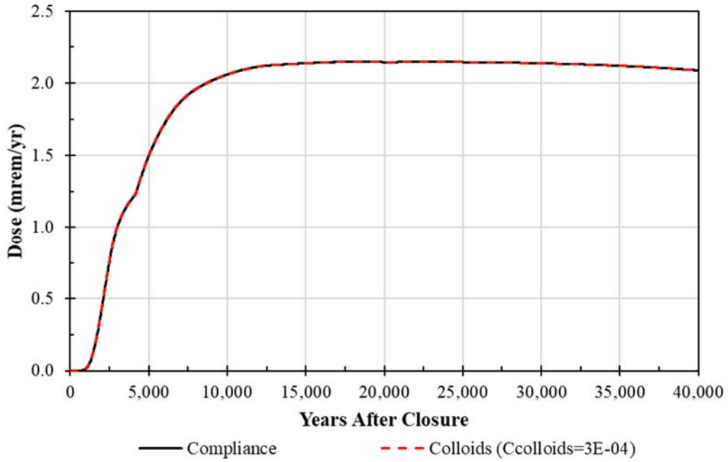
Figure 5.8-117: Comparison of Colloid Sensitivity Case ( C_{\text{colloids}}=3\text{E-}04 g/mL) Total Dose Results with Compliance Case Total Dose Results over 40,000 Years
