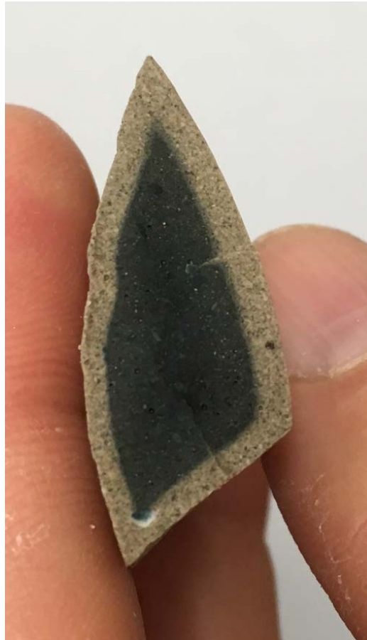
Figure A-6: Oxidation Front Penetrating a “Cement-Free” Saltstone Simulant Sample, Evident from Color Change
