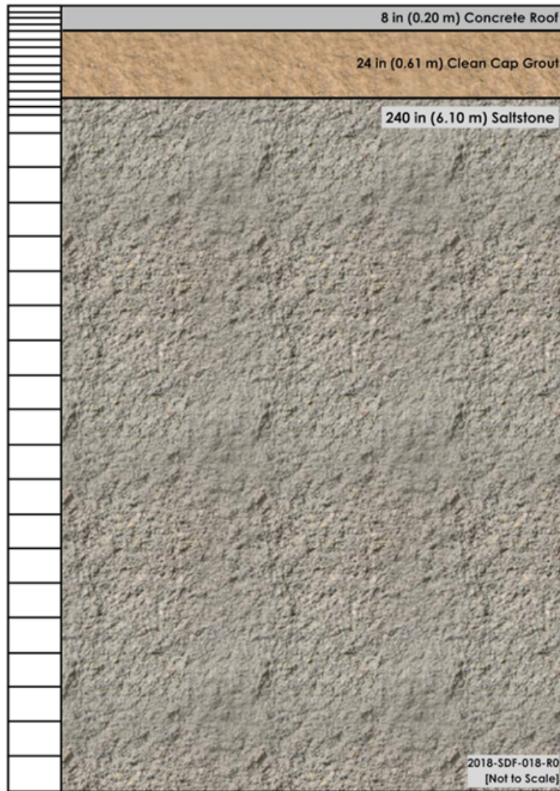
Figure 4.4-159: Schematic of the SDF APR Model Material Zones and Grid for Air and Radon Pathway Analyses for 150-Foot Diameter SDUs
