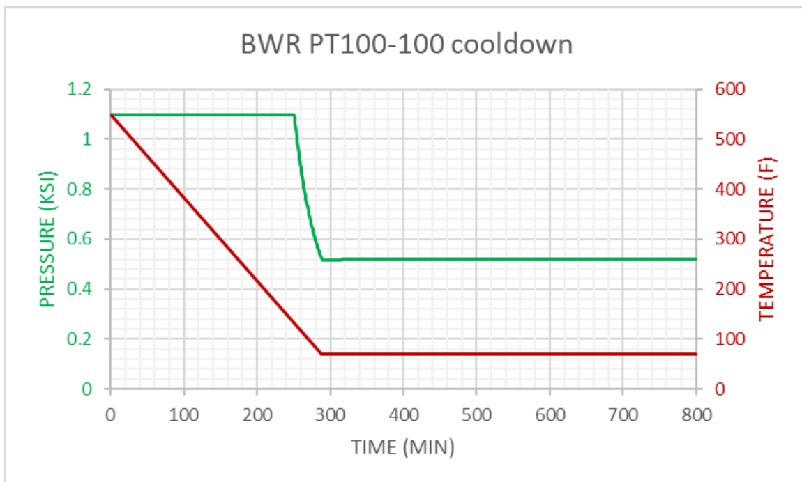
Figure 3-2: BWR PT100-100 Cooldown Transient Characteristics
