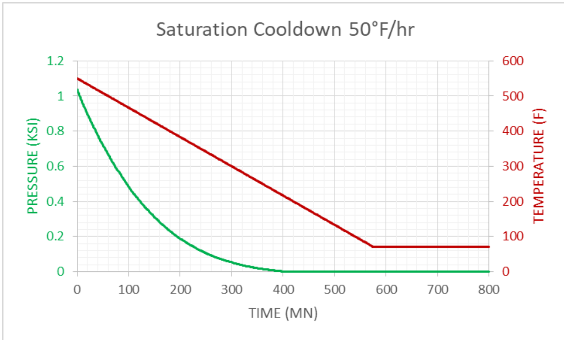
Figure 3-5: BWR Saturation Cooldown at 50°F/hour Transient Characteristics
