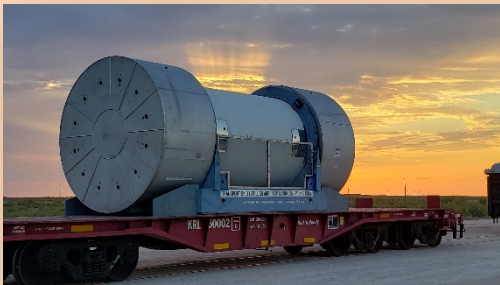
Type B MP197HB spent fuel package on a transport vehicle. Photo courtesy © Orano.
