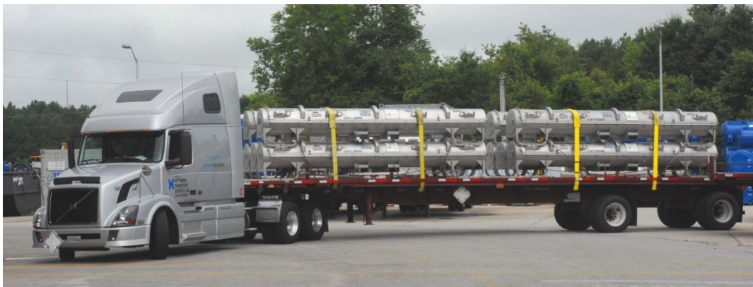
23 24 Figure 3-25 Ten Traveller Unirradiated Fuel Transportation Packages Being 25 Transported on a Truck (Source: Photo provided by the WEC).
