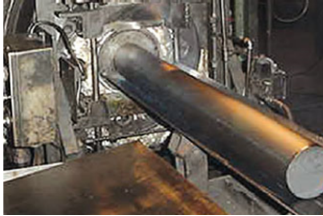
Figure 3-19 Graphite extrusion exiting from the die. Image courtesy of NAC carbon, NAC Carbon Products, in Punxsutawney, PA
