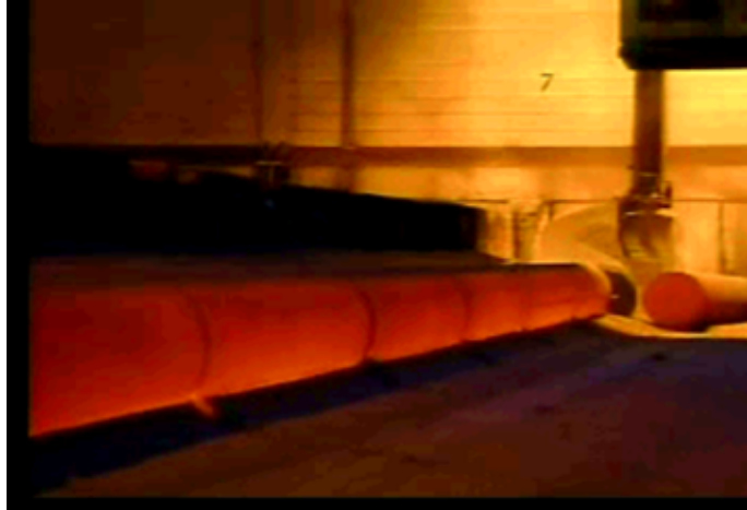
Figure 3-28 Longitudinal furnace graphitization operation, from Burchell (2018). Image courtesy of Richard W. Barnes, President, ANRIC
