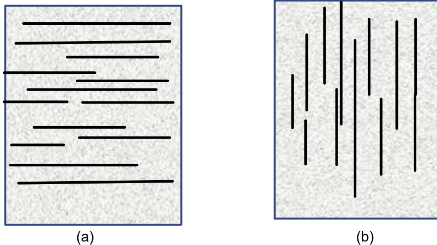
Figure 4-4 (a) All cracks are formed perpendicular to the wall surface; (b) all cracks are formed parallel to the wall surface
