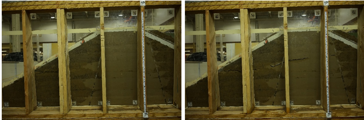
Figure 5-2 Pipe beginning to develop through embankment after removal of rebar on second day of testing. Elapsed times since the restart on the second day are 1 min (left) and 103 minutes (right). In the first photo the pipe is only visible in the downstream gravel zone. In the right hand photo, the color variation in the portion of the pipe within the core zone indicates redeposition of soil in the bottom of the pipe as erosion occurs from the roof.
