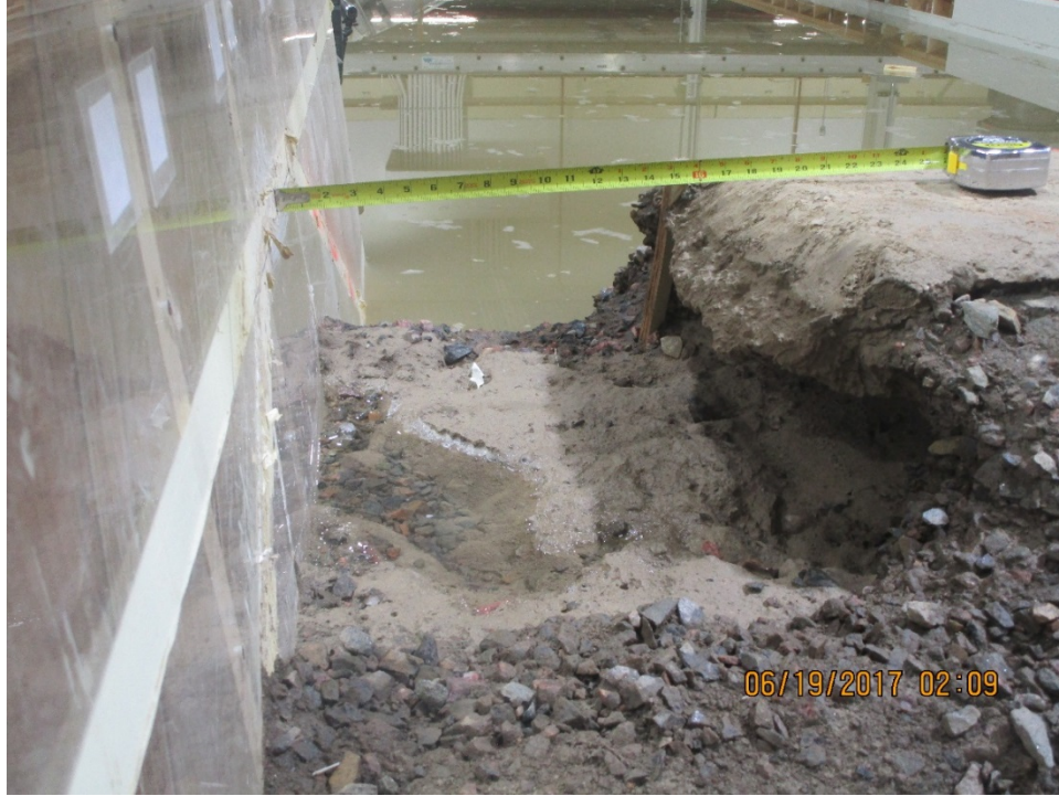
Figure 4-2 Breach pilot channel at the end of the first day of testing. Note the embedded wood stake that appeared to restrict lateral erosion.
