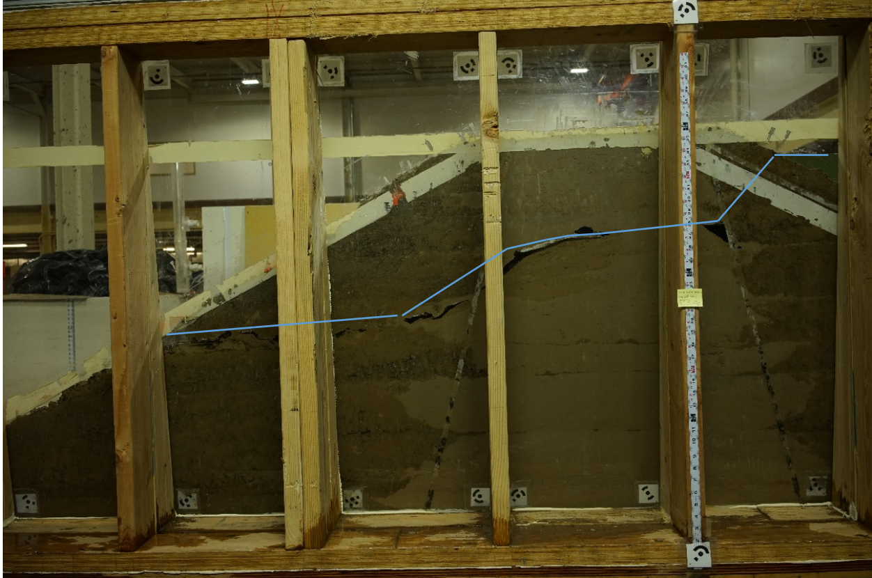
Figure 5-3 Development of stepped profile of erosion channel. An approximate hydraulic grade line for the flow is sketched over the photo in blue. As the roof of the channel collapsed and the bed migrated upward, most of the core zone began to experience open-channel, rather than pressurized flow.
