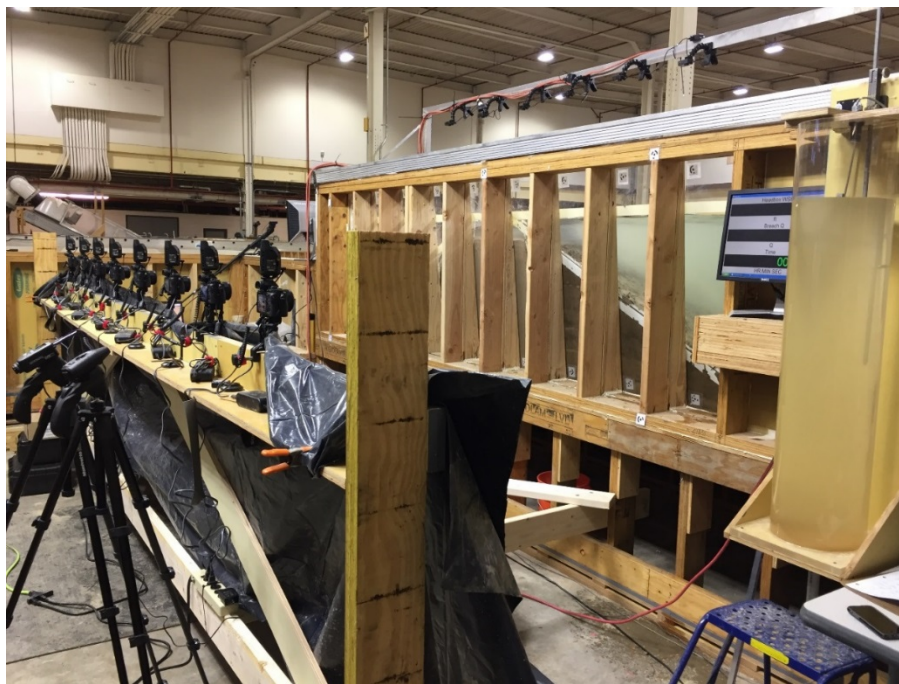
Figure 2-3 Camera equipment used during the test included six GoPro cameras deployed above the embankment and eight DSLR cameras viewing the left abutment through the acrylic wall.
