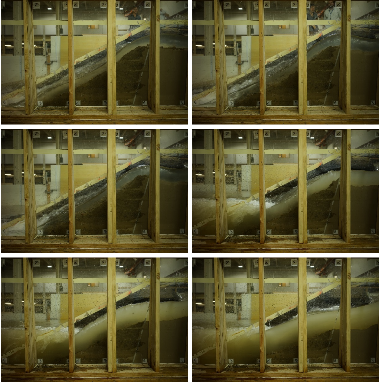
Figure 4-6 Photos of breach channel downward erosion progress on the second day of the zoned embankment overtopping test. Total elapsed times in minutes in the photos from left-to-right, top-to-bottom are: 34.5, 37, 47, 77, 120, 180.
