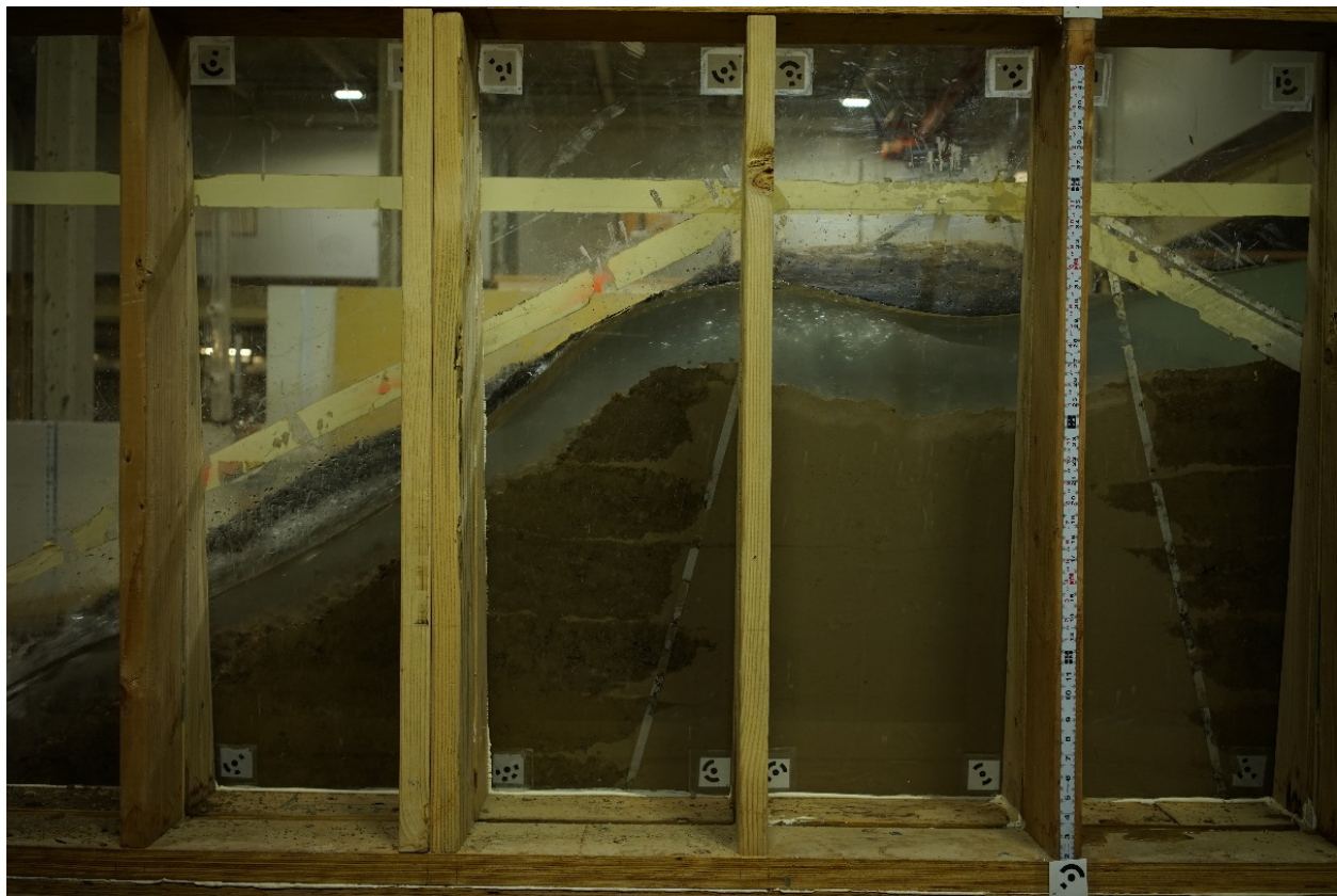
Figure 4-1 Erosion of top surface of core zone after about 6 minutes of flow on the second day of testing.
