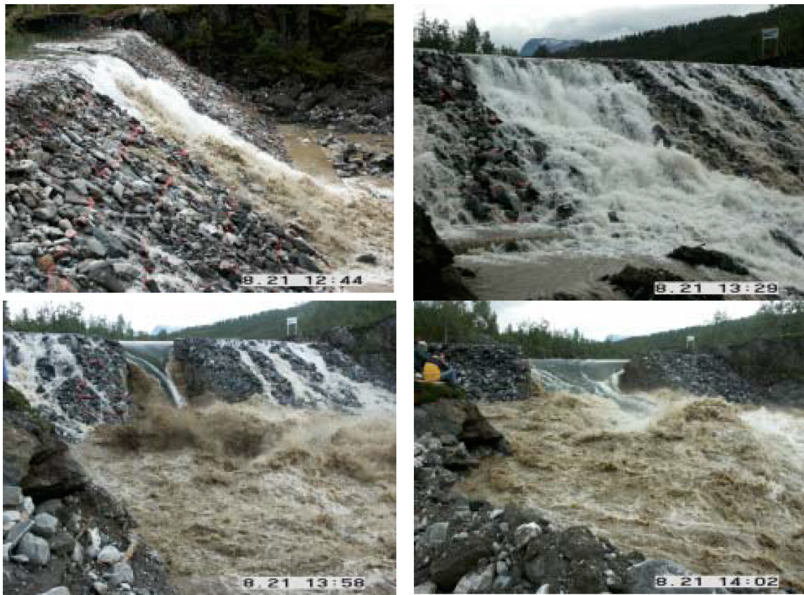
Figure 6-5 Headcut development during IMPACT test of zoned gravel dam, 1-2003 (from IMPACT WP2 Technical Report: Section 4).
