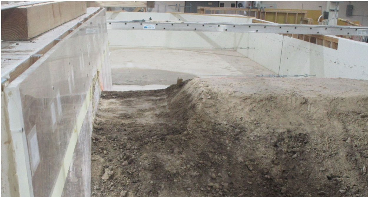
Figure 2-7 Pilot channel in zoned embankment prior to overtopping test.
