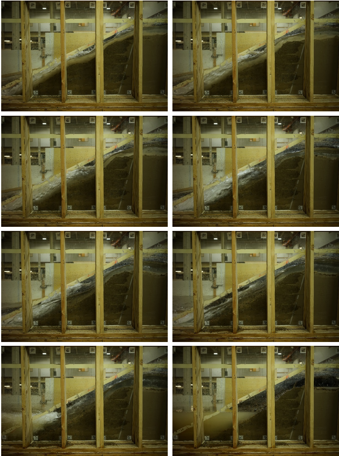
Figure 4-5 Photos of breach channel downward erosion progress on the first day of the zoned embankment overtopping test. Elapsed times (mm:ss) in the photos from left-to-right, top-to-bottom are: 3:20, 5:20, 7:20, 14:20, 19:20, 26:20, 33:20, and 33:20 (after flow was stopped).
