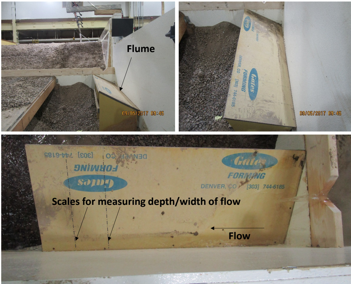
Figure 2-2 Supercritical flume downstream from left edge of embankment. The bottom photo is taken from directly overhead and shows the scales used to indicate the depth and width of flow, which were correlated to flow rate through in-place calibration.
