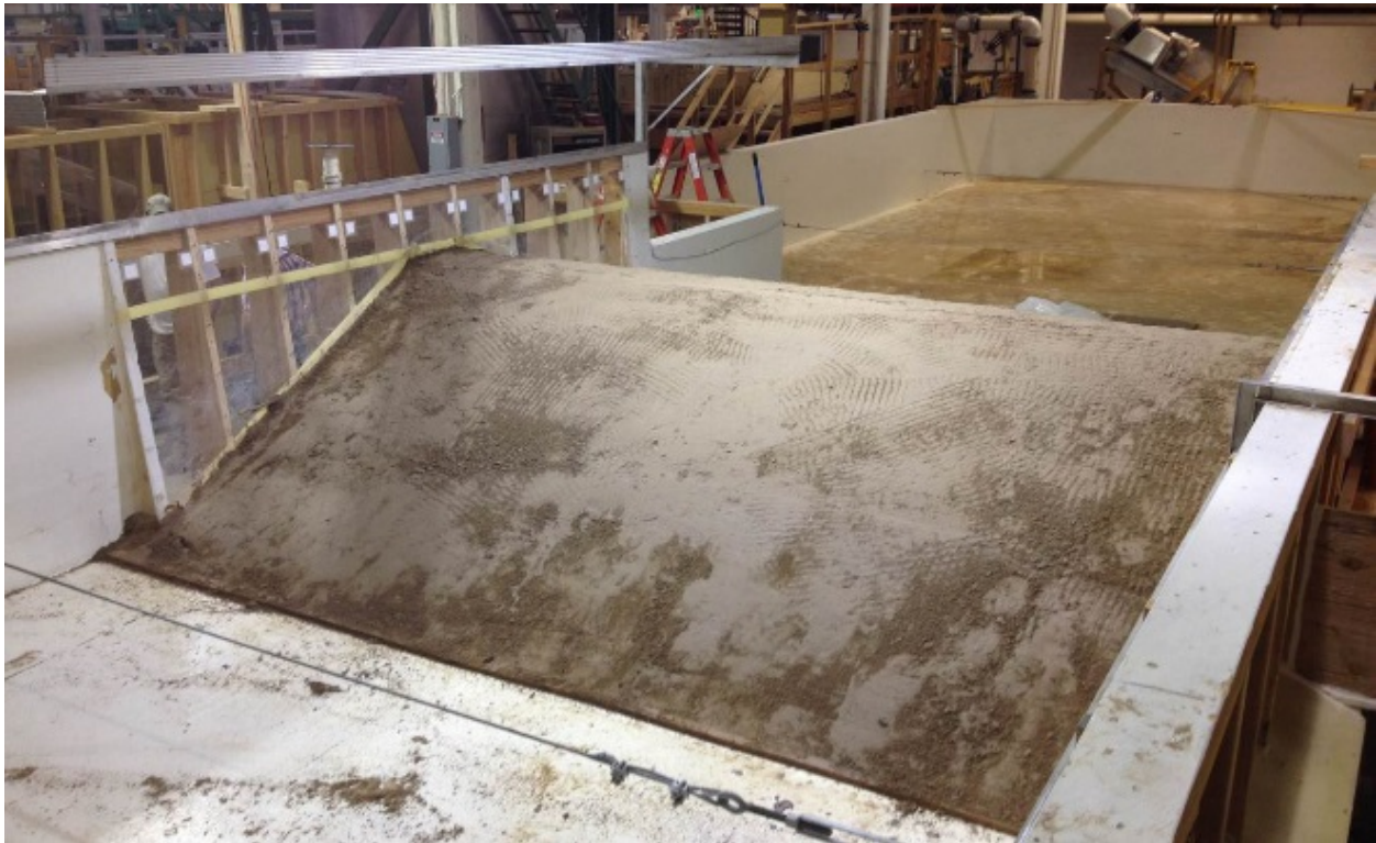
Figure 2-1 Embankment breach test facility viewed from the upstream end of the headbox, overlooking the homogeneous CL-ML embankment (Dam Safety-funded first test).
