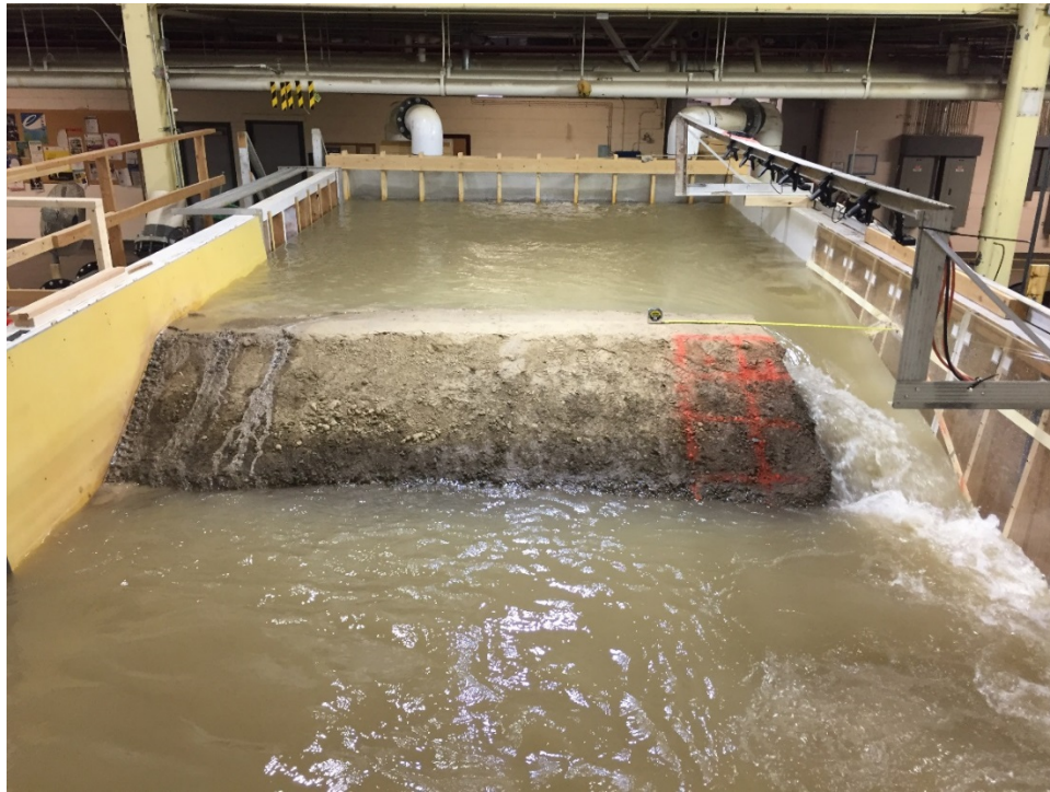
Figure 4-3 Flow conditions through the breach channel near the end of the zoned embankment overtopping test (t=2 hr 56 min).
