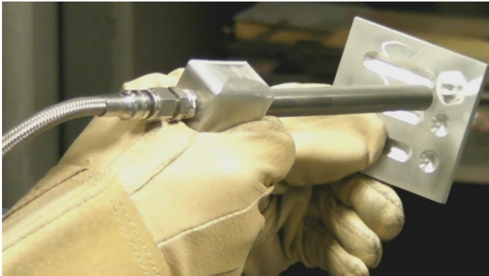
Figure 2-5 Handheld CS nozzle for small area application (courtesy of ARL).
