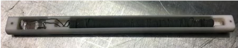
Ceramic enclosure housing sensor components
