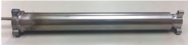
SS enclosure holds ceramic enclosure within autoclave PWR loop
