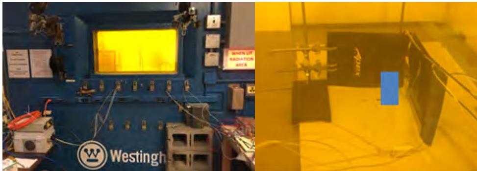
Gamma testing: Clean Hot Cell exterior (left) and interior (right)
