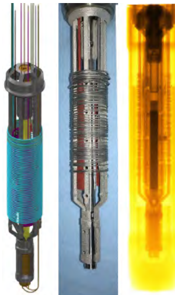
Instrumented capsule for LWR fuel safety test in TREAT
