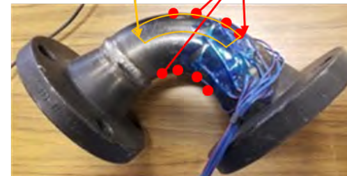
Printed SAWs developed and fabricated at ORNL – courtesy of Tim McIntyre
