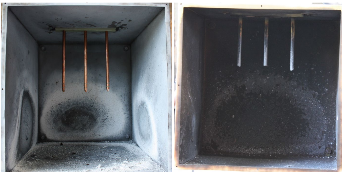
Fig. 40. Experiment OB09 pre-experiment (left) and post-experiment (right) copper electrodes. Phase sequence from left-to-right is C-B-A.
