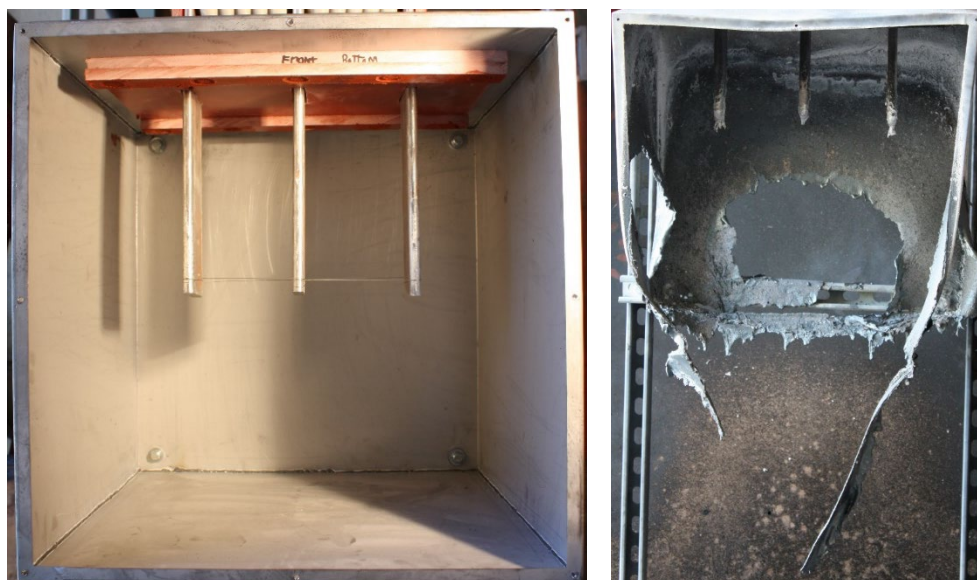
Fig. 73. Experiment OBMV06 pre-experiment (left) and post-experiment (right) aluminum electrodes. Phase sequence from left to right is C-B-A.
