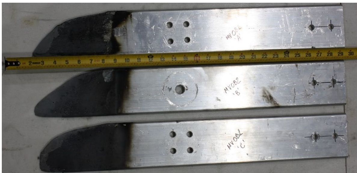
Fig. 65. Experiment OBMV02 aluminum electrodes post-experiment.
