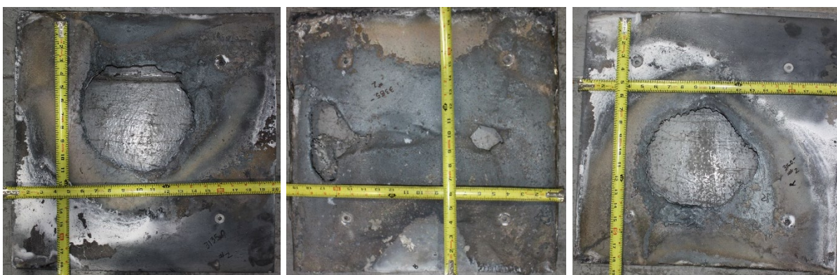
Fig. 64. Experiment OBMV2 enclosure breach (Left-to-right: left side, bottom side, right side).
