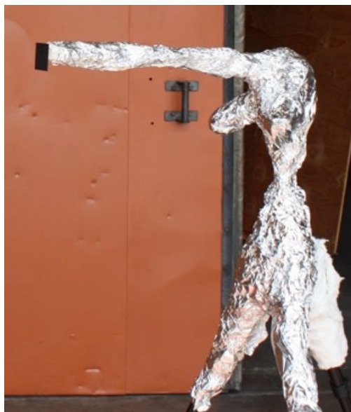
Fig. 10. Plate calorimeter apparatus in its thermal protected configuration.
