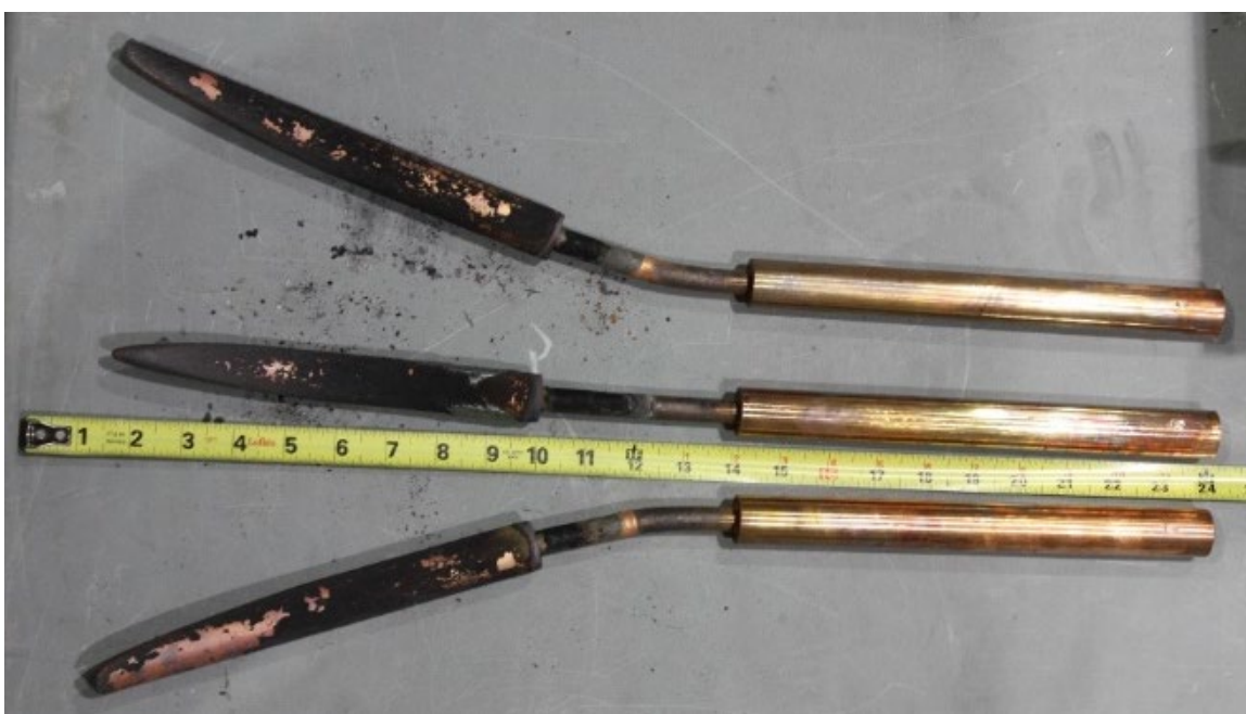
Fig. 38. Experiment OB04 electrode deflection post-experiment.
