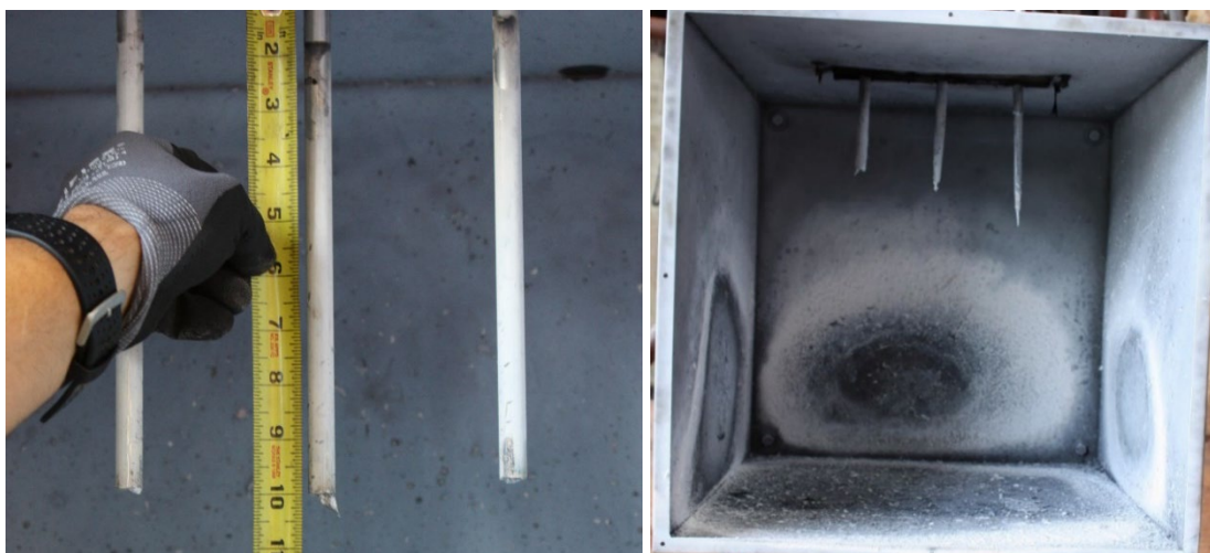
Fig. 52. Experiment OB10 pre-experiment (left) and post-experiment (right) aluminum electrodes. Phase sequence from left-to-right is C-B-A.
