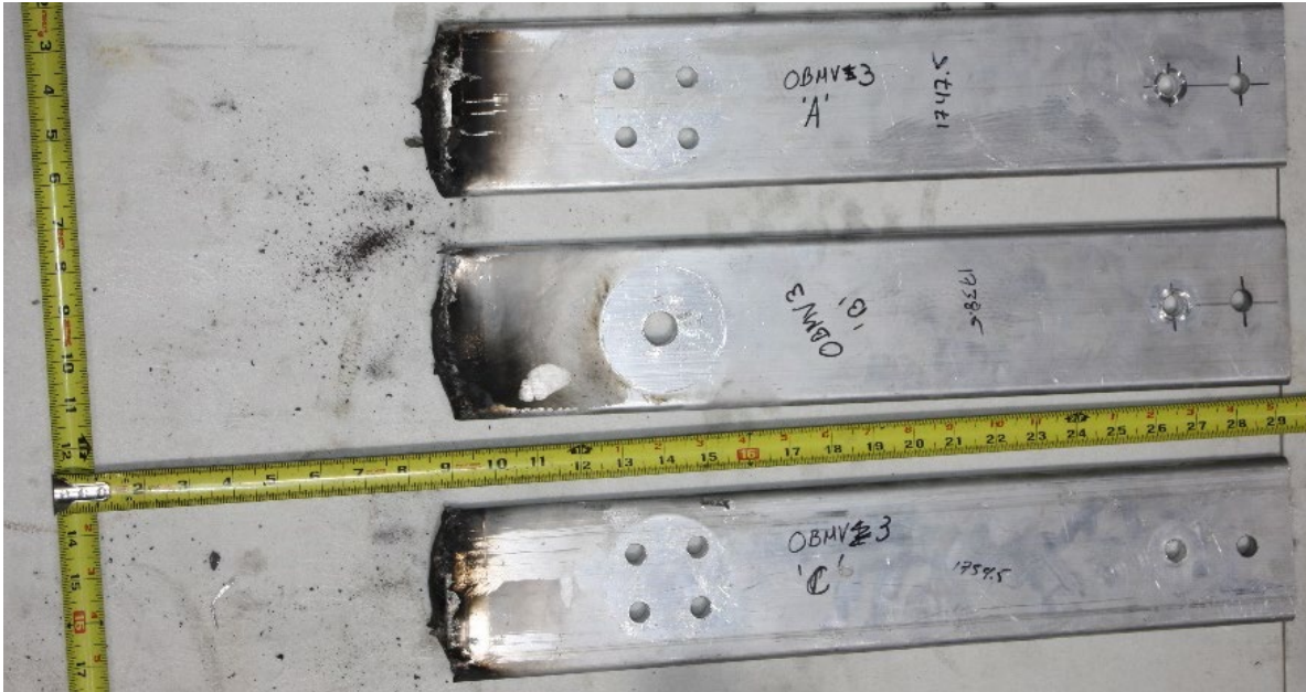
Fig. 71. Experiment OBMV03 aluminum electrode post-experiment.
