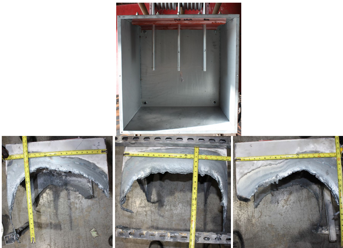
Fig. 60. Experiment OBMV01 pre-experiment (top) and post-experiment (left side (bottom left), back (bottom center), right side (bottom right)). Phase sequence from left to right is C-B-A.
