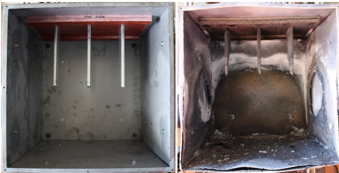
Fig. 63. Experiment OBMV02 pre-experiment (left) and post-experiment (right) aluminum electrodes. Phase sequence from left to right is C-B-A.
