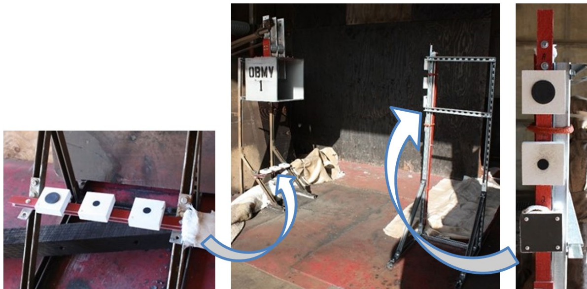
Fig. 14. Calorimeter arrays used during medium-voltage experiments (horizontal array (left), array location within cell (center), vertical array (right)).
