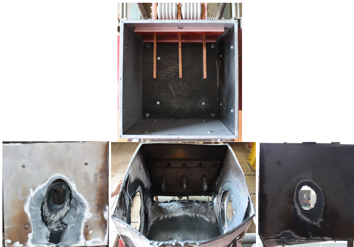
Fig. 58. Experiment OBMV05 pre-experiment (top) and post-experiment (bottom, left-to-right, left side from outside, front, right side from outside). Phase sequence from left to right is C-B-A.
