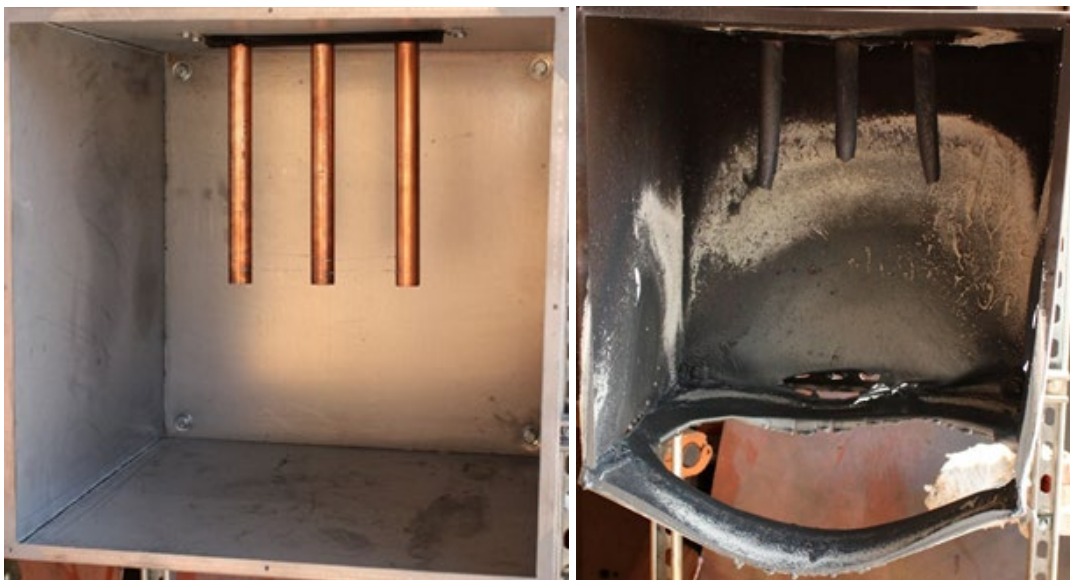
Fig. 33. Experiment OB03 pre-experiment (left) and post-experiment (right) copper electrodes. Phase sequence from left-to-right is C-B-A.
