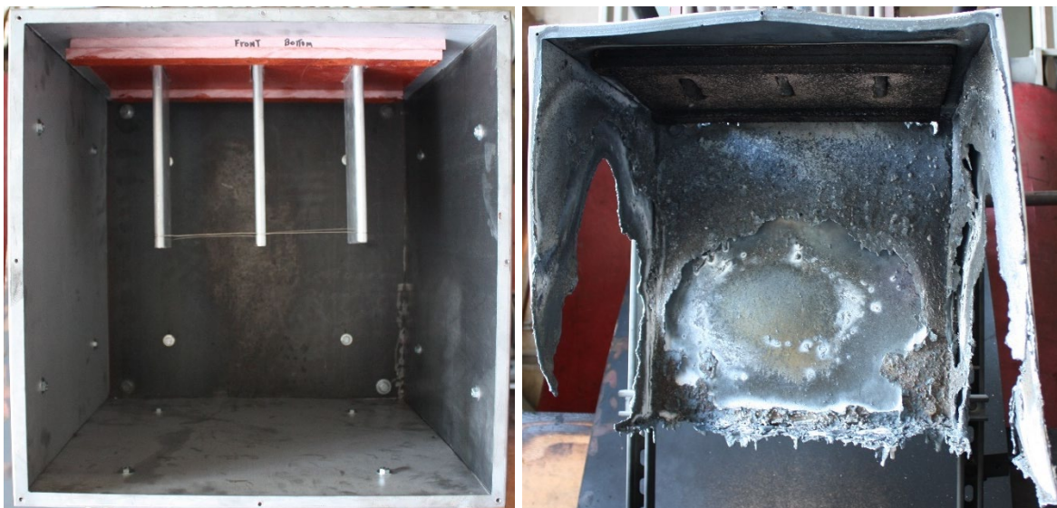
Fig. 69. Experiment OBMV03 pre-experiment (left) and post-experiment (right) aluminum electrodes. Phase sequence from left to right is C-B-A.
