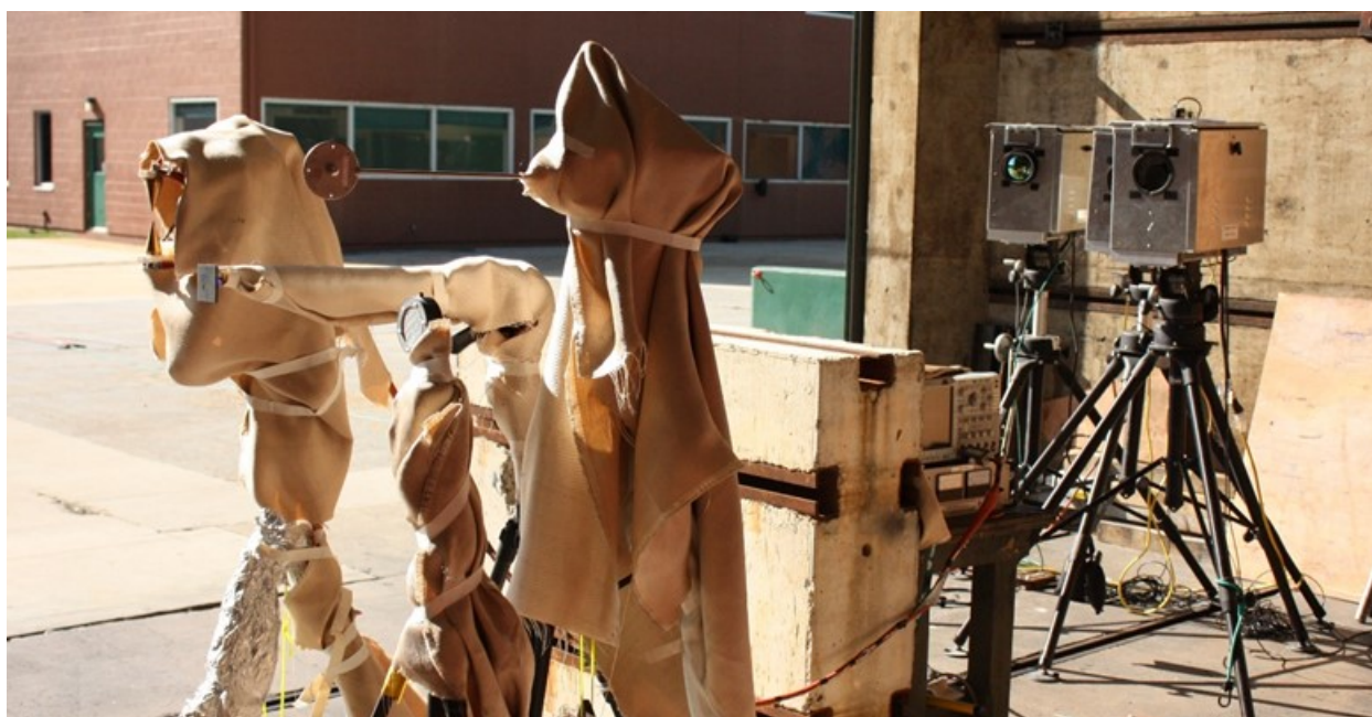
Fig. 6. Instrumentation cluster covered with heat resisting fabric for protection during experiments (from left-to-right, air breakdown, plate calorimeter, d-dot, air conductivity, high speed IR, and visible videography).
