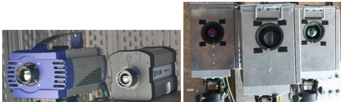
Fig. 9. Thermal imagers used inside and outside the test cell (thermal imaging cameras located approximately 27 m from the open box (left), imaging cameras located within the test cell (right), from left to right: thermal, high speed visible, thermal).
