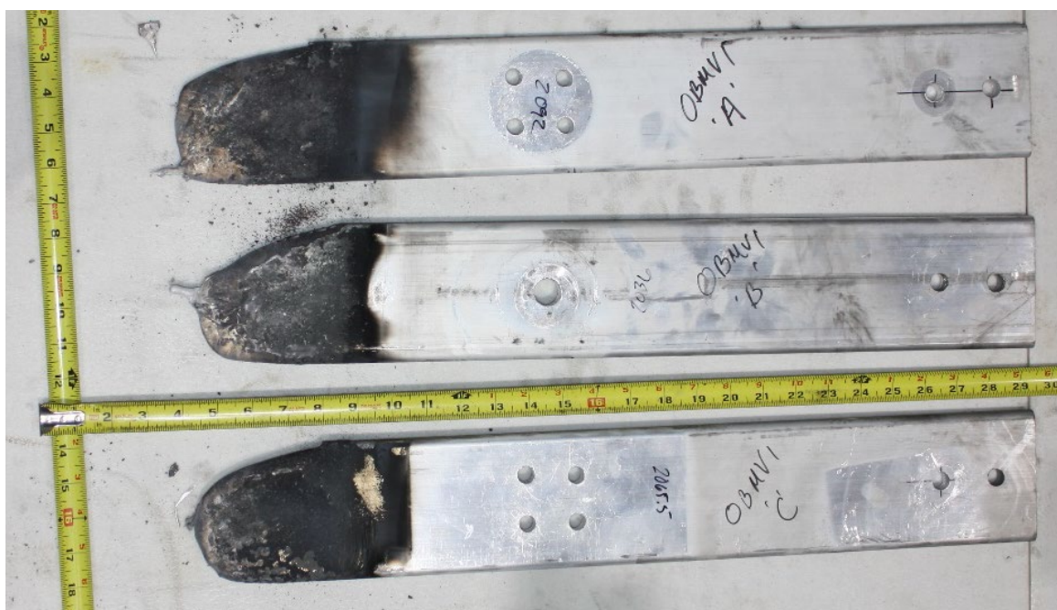
Fig. 61. Experiment OBMV01 aluminum electrode post-experiment.
