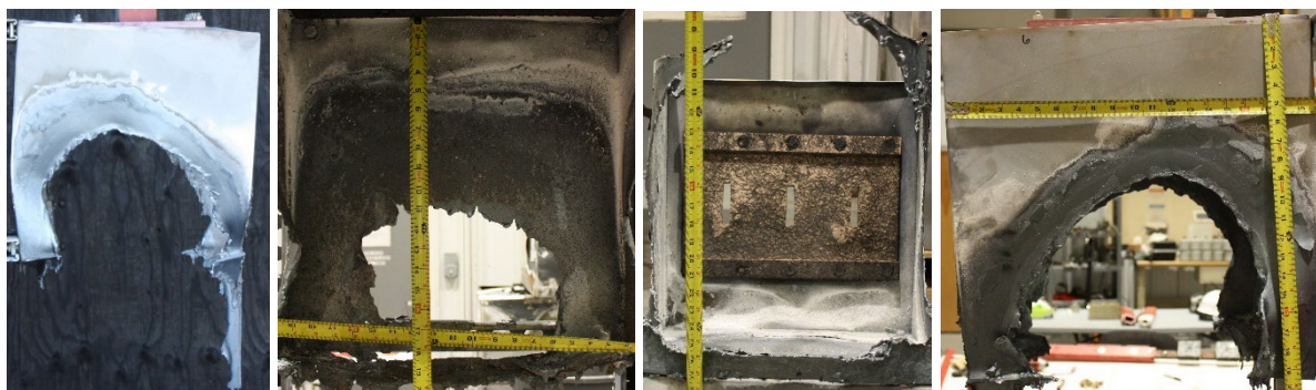
Fig. 74. Experiment OBMV6 enclosure breach (Left-to-right: left side, back side, bottom side, and right side).
