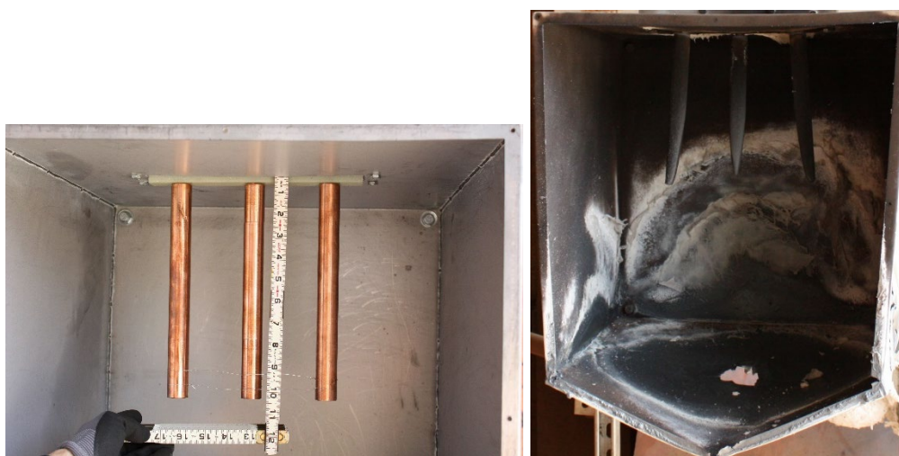
Fig. 36. Experiment OB04 pre-experiment (left) and post-experiment (right) copper electrodes. Phase sequence from left to right is C-B-A.
