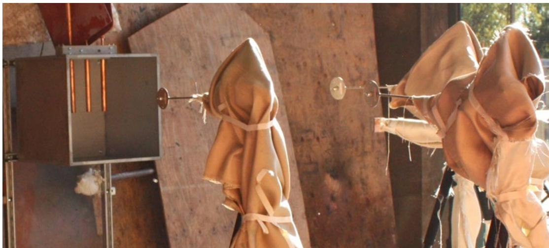
Fig. 17. d-Dot sensors arrangement prior to experiment. Note all sensors oriented in same axis based on results from earlier experiment indicating the largest measured signal.
