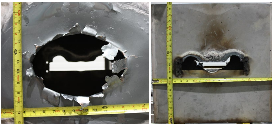
Fig. 31. Experiment OB02 enclosure breach. (bottom side breach (left), top side breach with electrode holder removed (right)).
