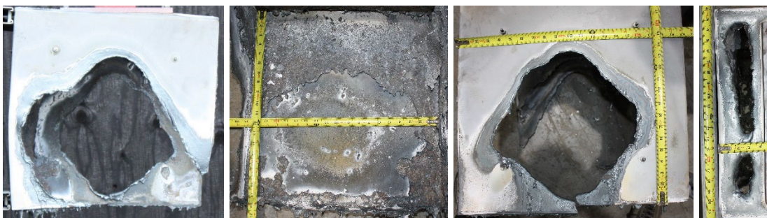
Fig. 70. Experiment OBMV03 enclosure breach (left-to-right: Left side, back side, right side, top).
