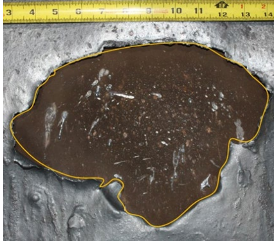
Fig. 22. Example of mass loss measurement using surface area estimated by computer software (363 cm 2 estimated area in example photo shown).
