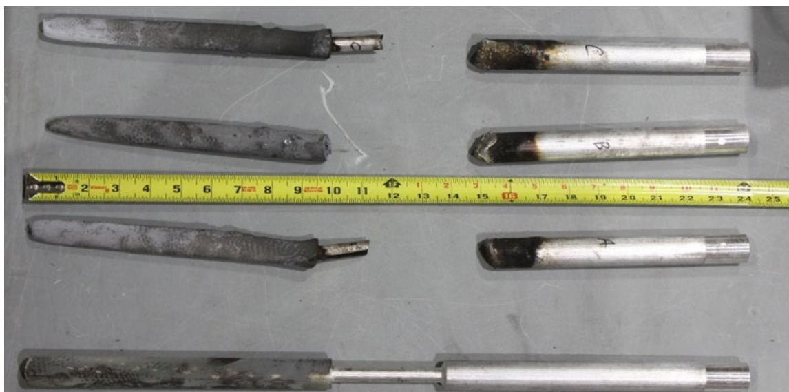
Fig. 51. Experiment OB08 aluminum electrodes post-experiment (top three, bottom electrode is from another experiment and included for comparison).
