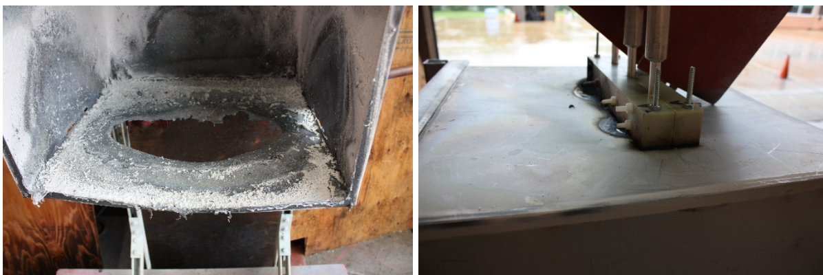
Fig. 47. Experiment OB07 enclosure breach (bottom and sides (left); rear top side (right)).
