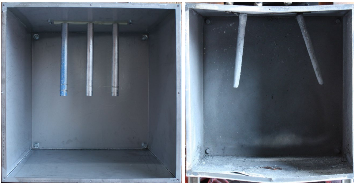
Fig. 49. Experiment OB08 pre-experiment (left) and post-experiment (right) aluminum electrodes. Phase sequence from left-to-right is C-B-A. Note the center electrode was ejected free from the box during the experiment.
