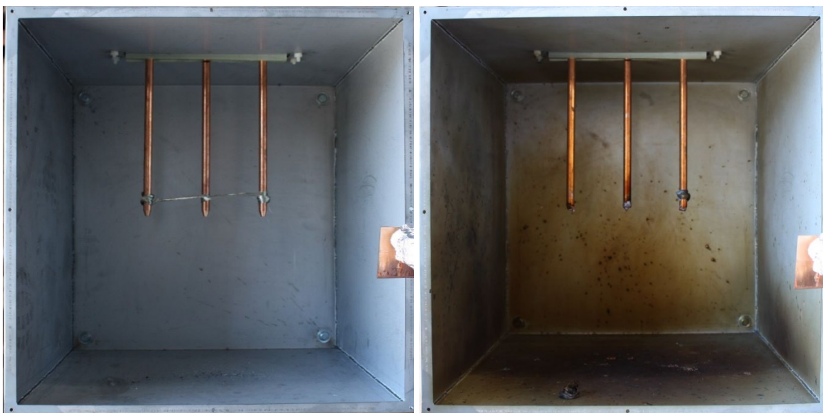
Fig. 27. Experiment OB01(a) pre-experiment (left) and post-experiment (right) copper electrodes. Phase sequence from left-to-right is C-B-A.
