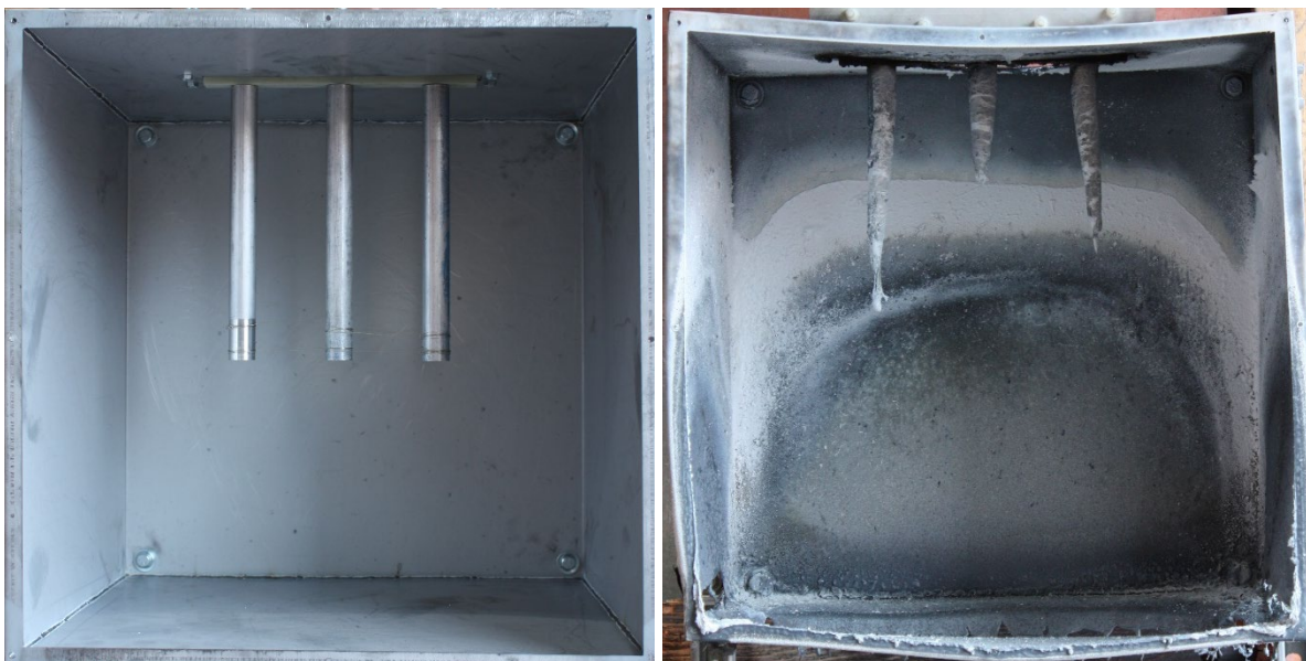
Fig. 44. Experiment OB06 pre-experiment (left) and post-experiment (right) aluminum electrodes. Phase sequence from left-to-right is C-B-A.
