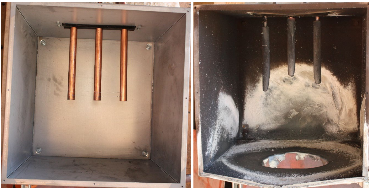
Fig. 30. Experiment OB02 pre-experiment (left) and post-experiment (right) copper electrodes. Phase sequence from left-to-right is C-B-A.
