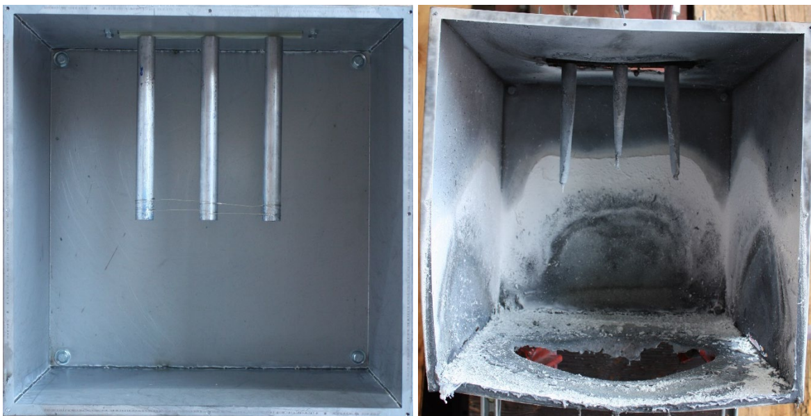
Fig. 46. Experiment OB07 pre-experiment (left) and post-experiment (right) aluminum electrodes. Phase sequence from left-to-right is C-B-A.
