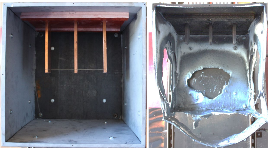
Fig. 55. Experiment OBMV04 pre-experiment (left) and post-experiment (right) copper electrodes. Phase sequence from left to right is C-B-A.
