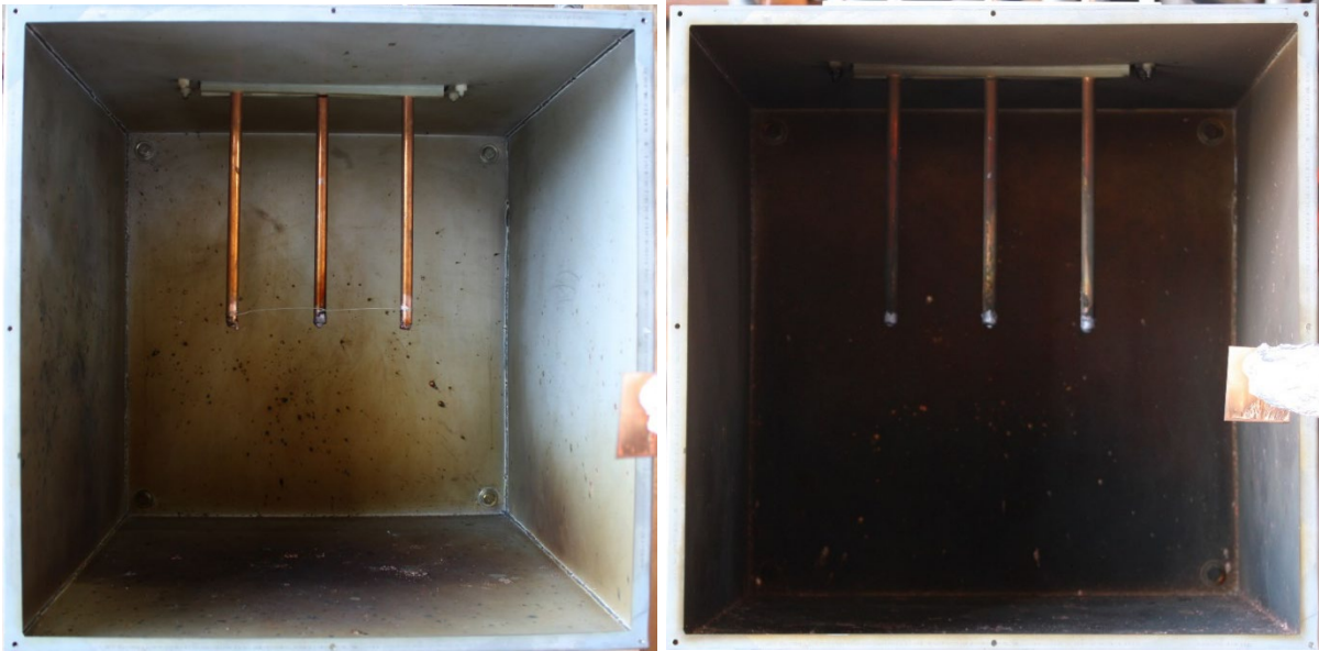
Fig. 29. Experiment OB01(b) pre-experiment (left) and post-experiment (right) copper electrodes. Phase sequence from left-to-right is C-B-A.
