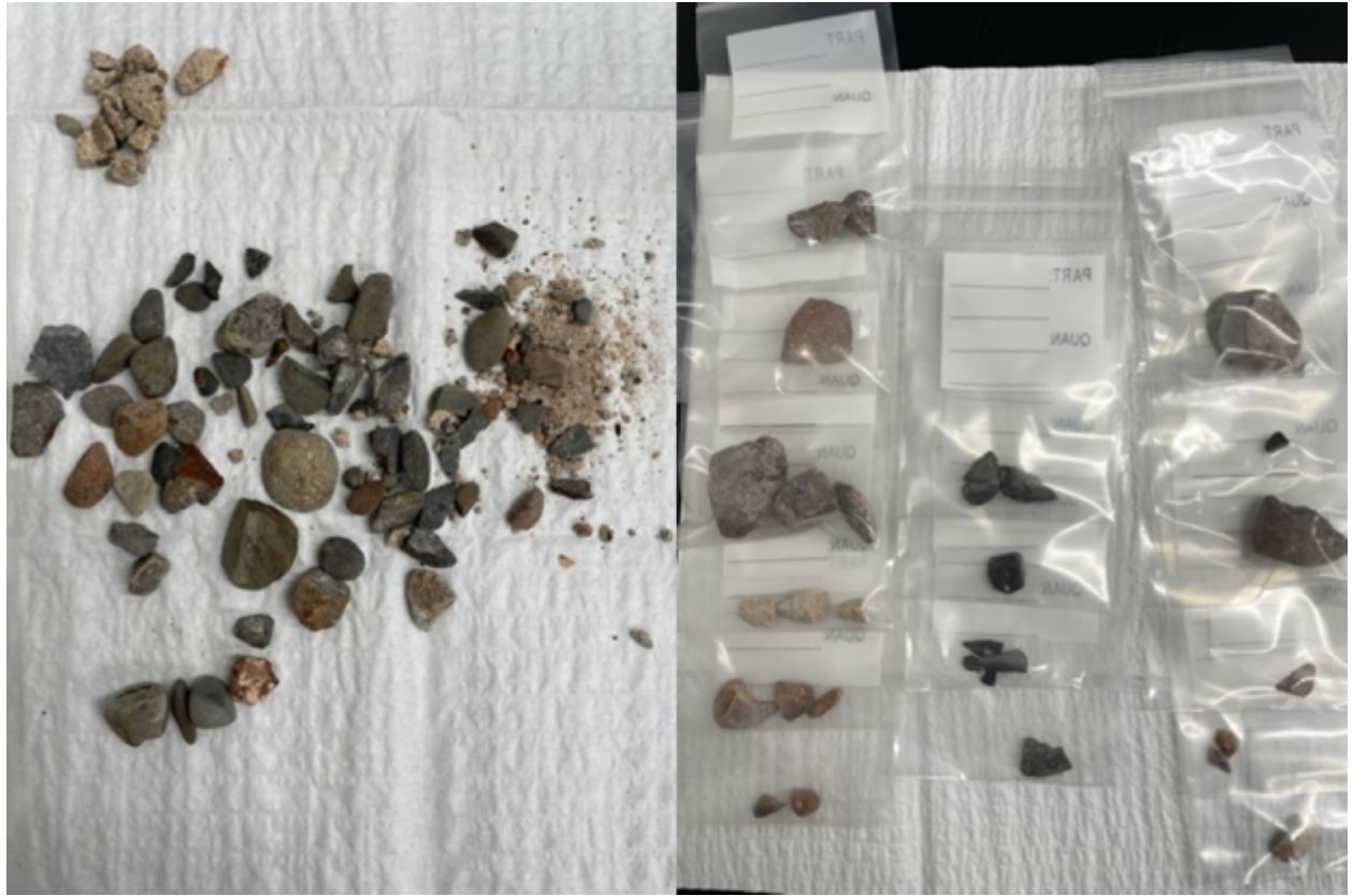
Figure 5-2 Aggregate separation for grinding and XRD analyses for mineral phase identification and quantification
