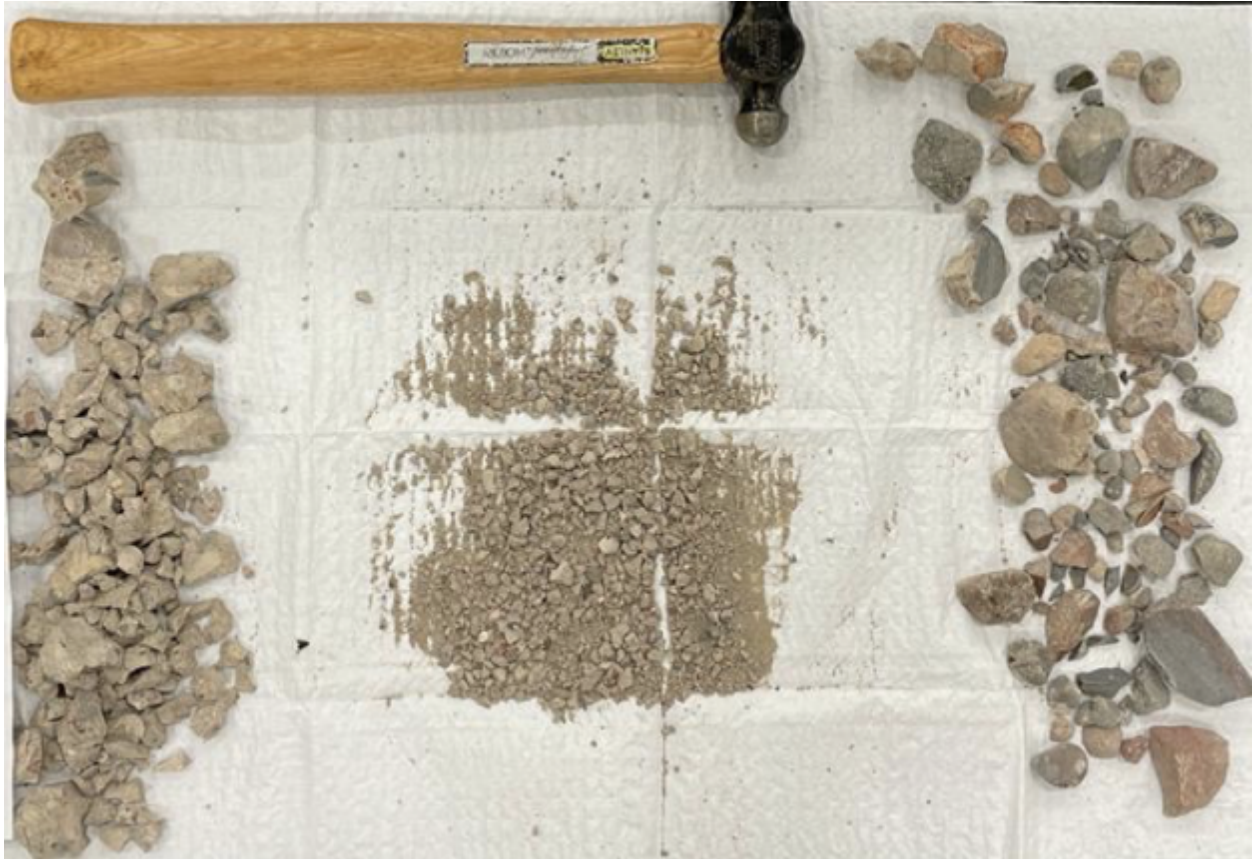
Figure 5-1 Resulting pieces of the core after heat and mechanical treatments
