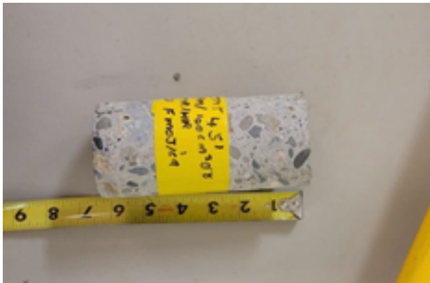
Figure 3-3 Cored specimen at 45 ft elevation
