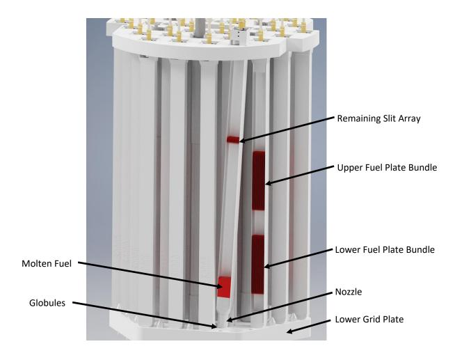
It is further assumed that the interaction of cooling water with the molten fuel that was kept molten (or at least very hot) in the lower part of the fuel element, since it was still undergoing a nuclear reaction,
