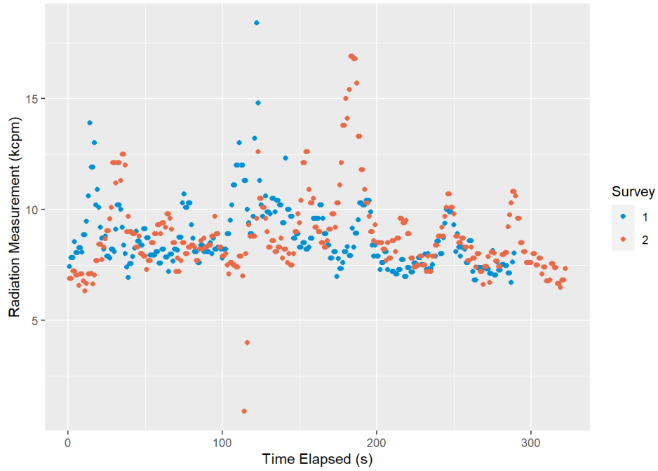
Figure E.33. Count Rates (kcpm) for Surveys 1 and 2 Over Time (s)
