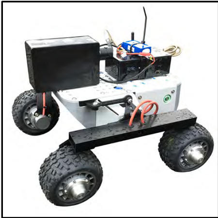
Figure 11-8 Kromek UGV Radiation Mapping RadRover
