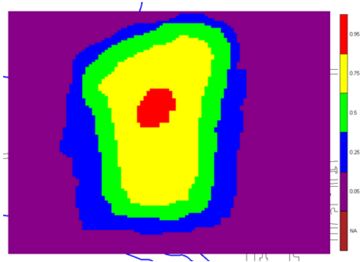
Figure 7-1 A User-Painted CCM Showing the User's Estimate of the Probability that the DCGL Will Be Exceeded in Samples across a Site as Shown in Color Scale
