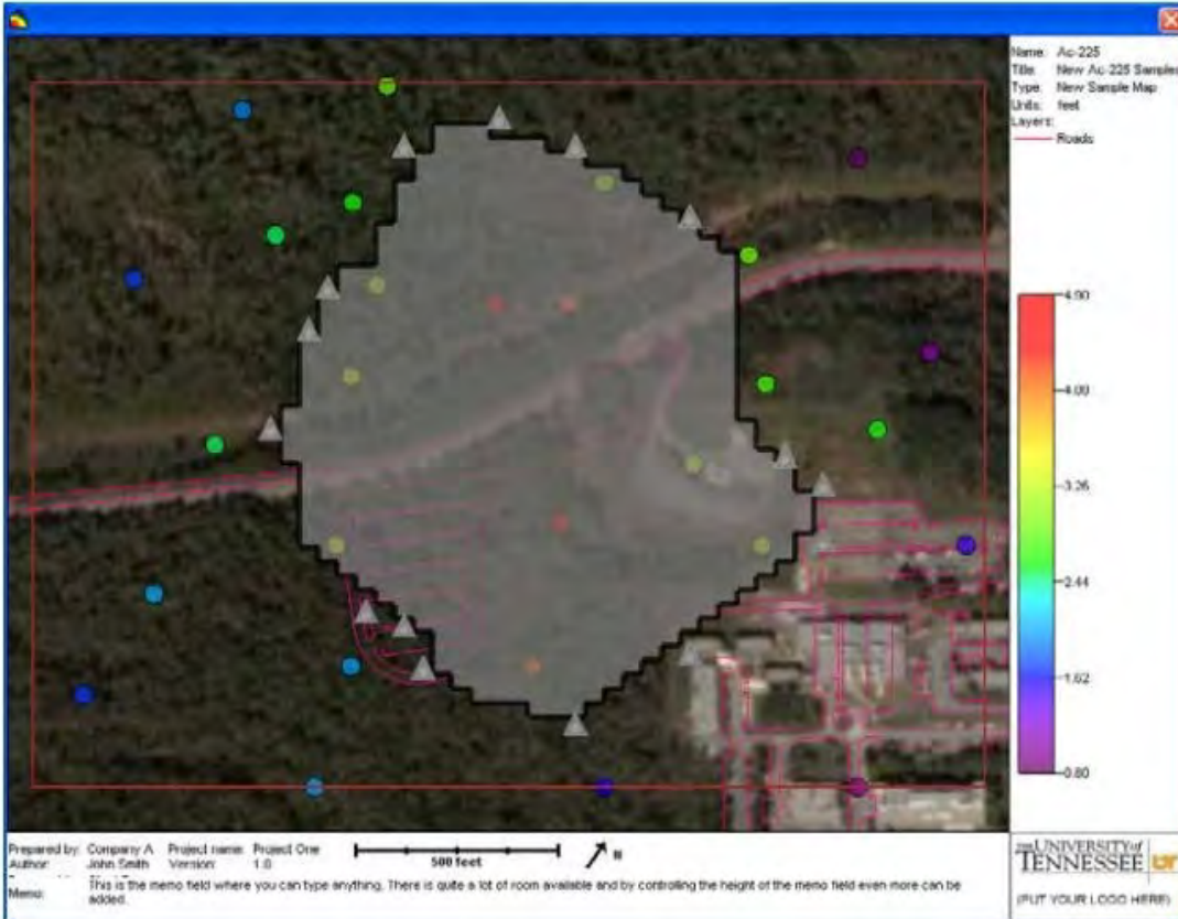
Figure B-3 Area of Concern Boundary Sampling Design in SADA (triangles indicate recommended samples)
