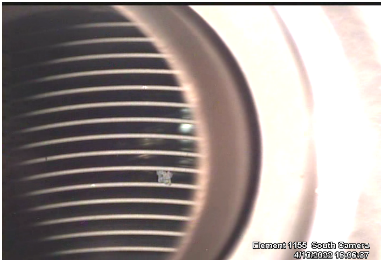
Figure 2. NIST personnel identified Element 1155 as likely containing fuel material.
