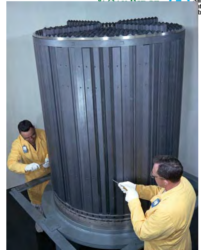
MSRE Graphite Core Structure [ https://en.wikipedia.org/wiki/Molten-Salt_Reactor_Experiment ]
