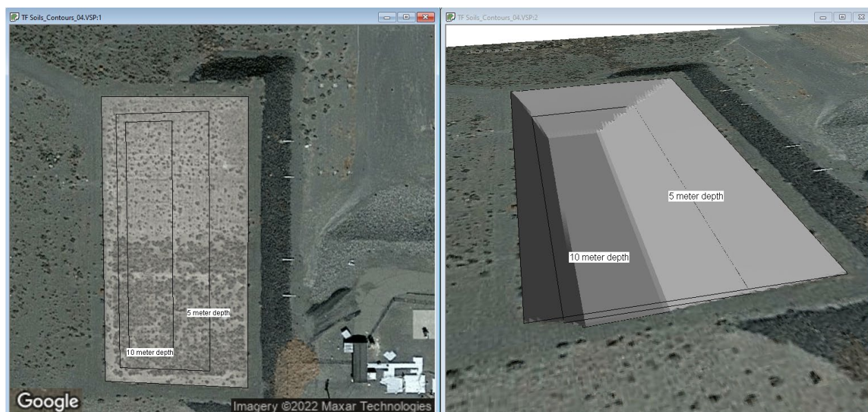
Figure 6. Example Volume Created with Rectangular Contours and Associated Depths. Contours are shown from above (left) and within the 3-D volume after applying the depths of each (right).
