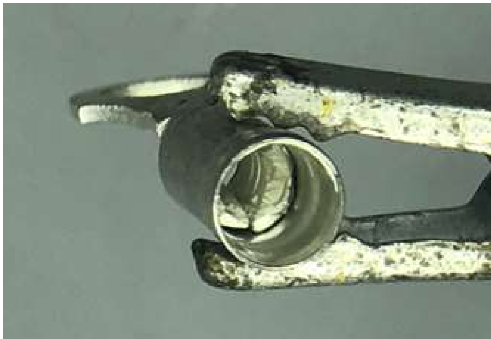
Photo # 7: Uncrimped Terminal with Blue Insulator Removed
