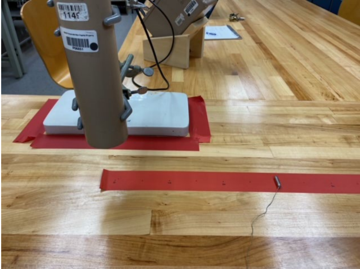
Figure 3.5. Offset experiment using a 4.76 \mu Ci Co-60 source
