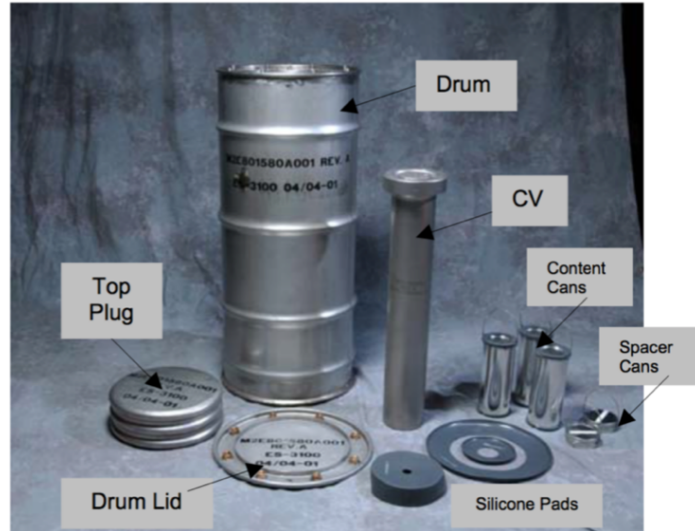
Figure 14. ES-3100 Type B shipping container [7].
