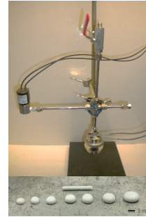
Batch-operated HR pneumatic salt sample generator
