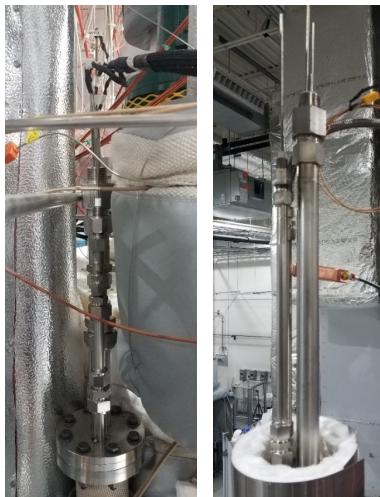
Multi-electrode array sensors installed onto the ORNL FASTR loop
