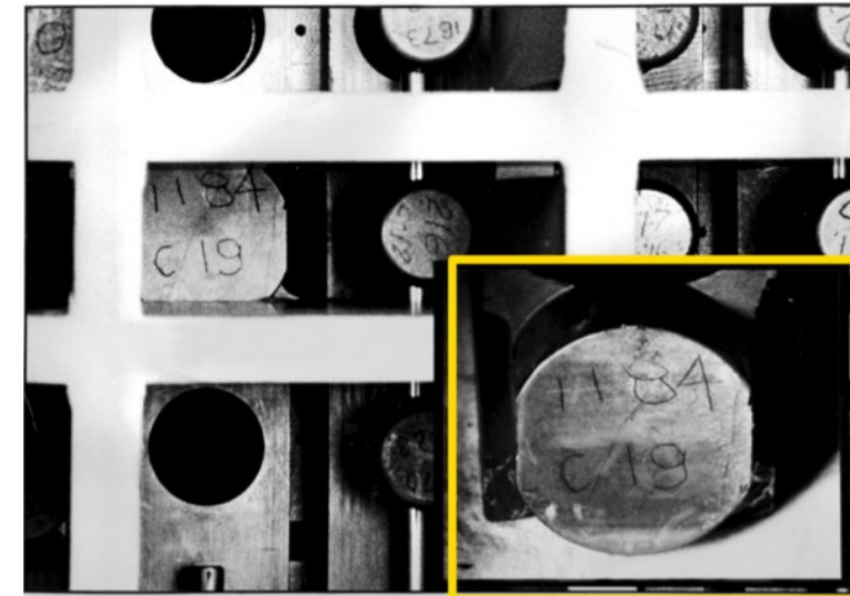
Bottom graphite stud of MSRE before (large photo) and after (inset) operation
