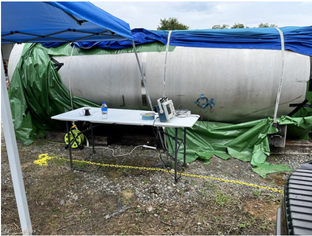
Transceiver placed in the exterior of the cask while sensor at same elevation inside cask
