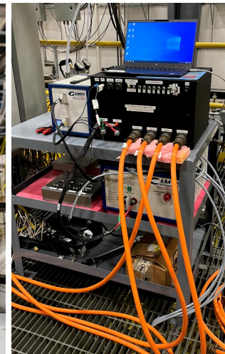
Instrumentation for distributed electrochemical sensors at the Kairo Power Engineering Test Unit
