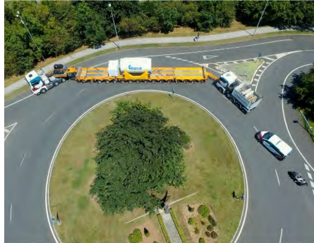
Road transport of a large spent fuel package
